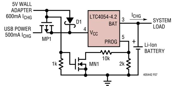
Figure 7. Combining Wall Adapter and USB Power
