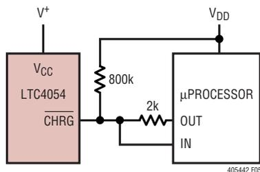
Figure 5. Using a Microprocessor to Determine  $\overline{\text{CHRG}}$  State
