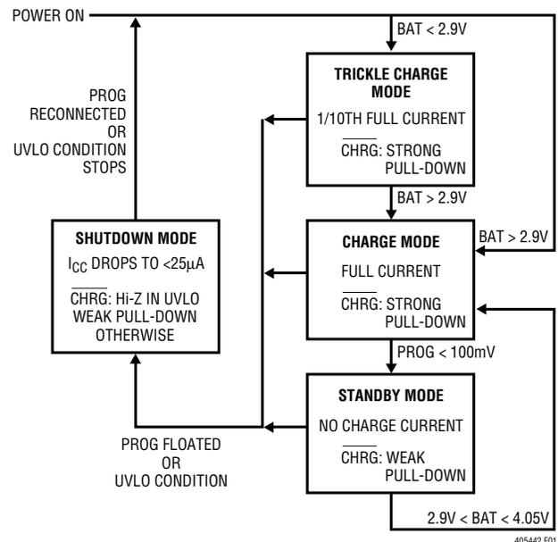
Figure 1. State Diagram of a Typical Charge Cycle
