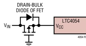
Figure 6. Low Loss Input Reverse Polarity Protection
