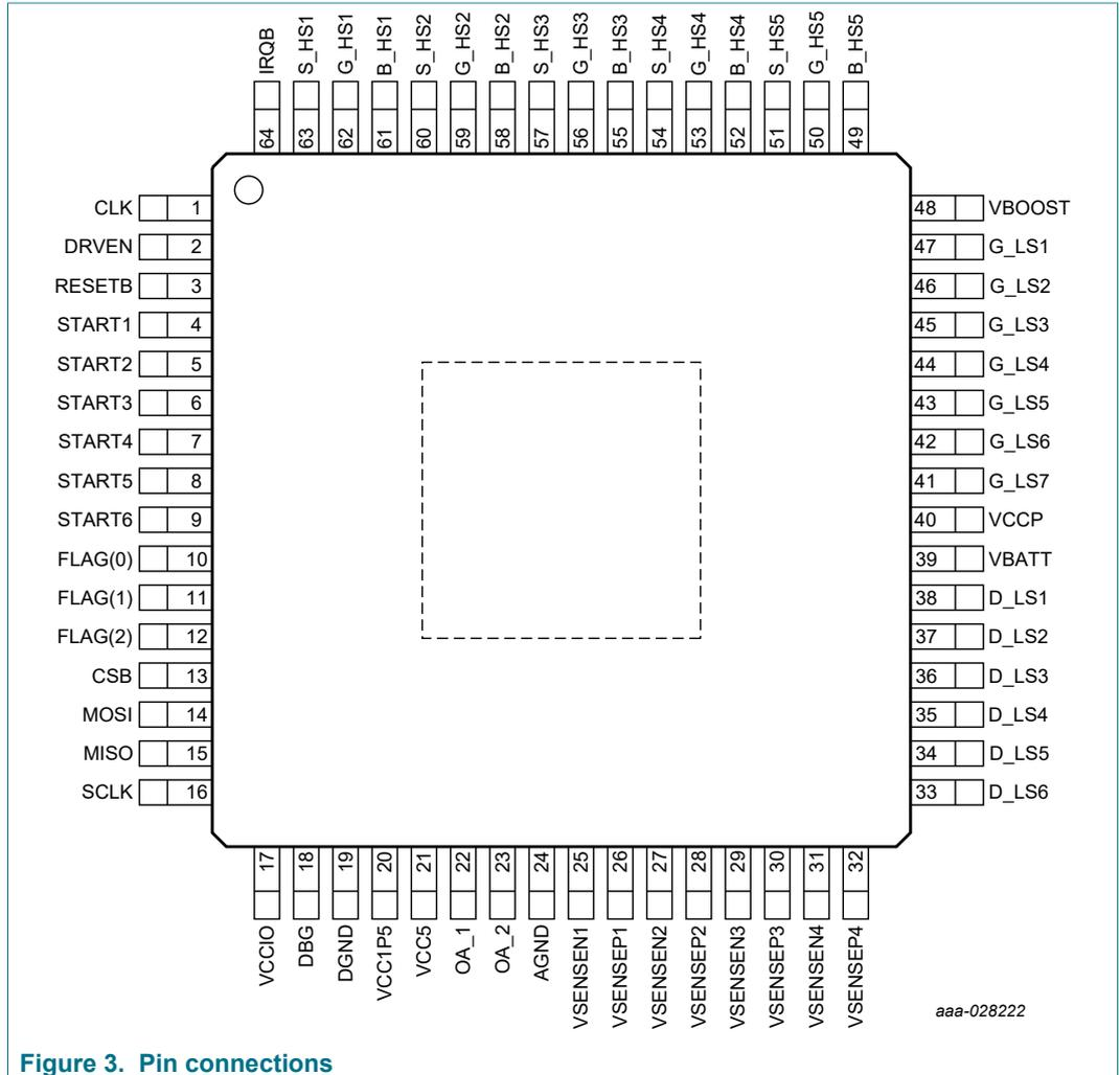
Figure 3. Pin connections
