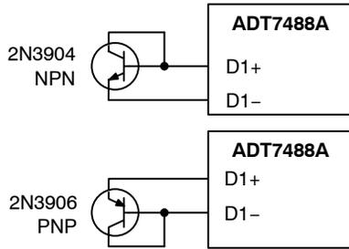
**Figure 16. Connections for NPN and PNP Transistors**
