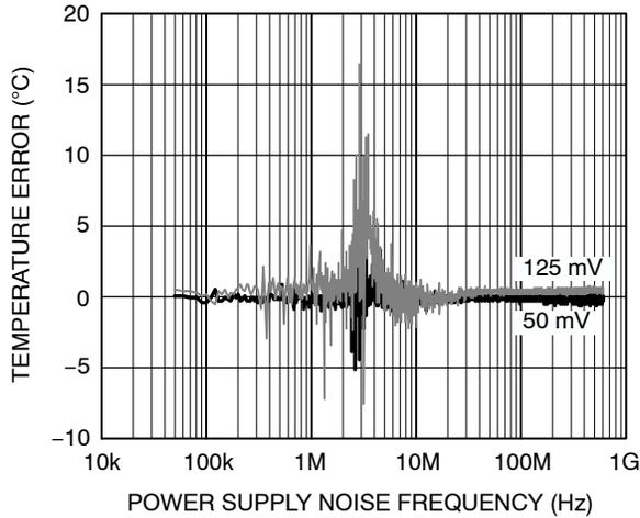
Figure 10. Local Temperature Error vs. Power Supply Noise
