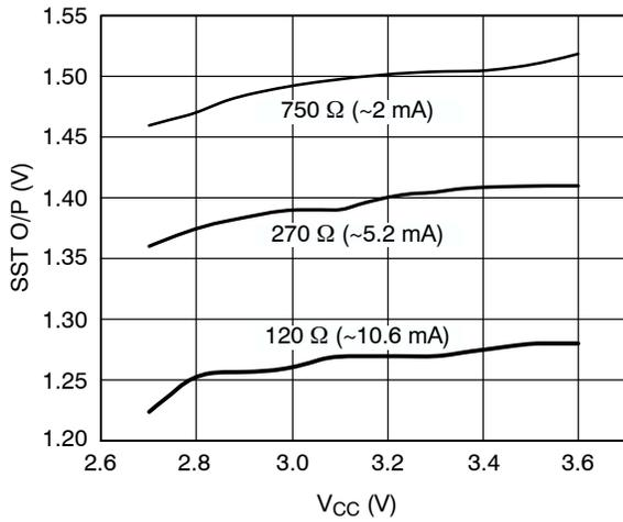
Figure 2. SST O/P Level vs. Supply Voltage
