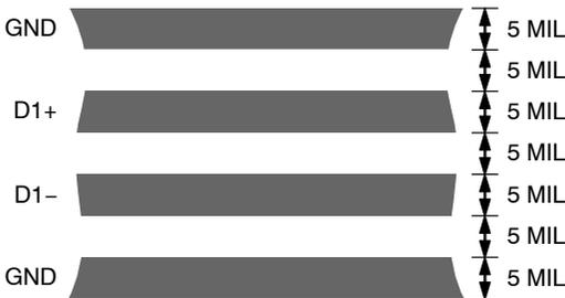
**Figure 17. Arrangement of Signal Tracks**
