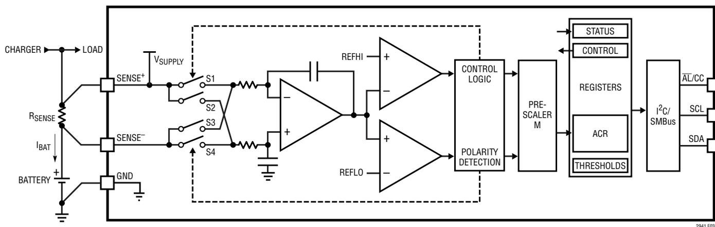
Figure 3. Coulomb Counter Section of the LTC2941
