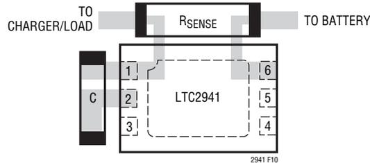
Figure 10. Kelvin Connection on Sense Resistor
