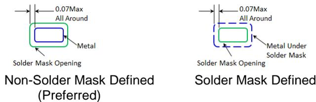
**Figure 11 Solder Mask Pattern**
