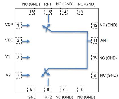
**Figure 2 Function Block Diagram**
