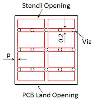
**Figure 14 Stencil Openings Shall not Cover Via Areas If Possible**
