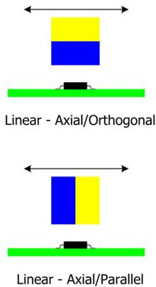
Linear Position Sensor with Axial Orthogonal Principle - 10 ... + 10 mm
