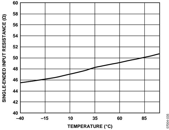
Figure 16. Single-Ended Input Resistance vs. Temperature
