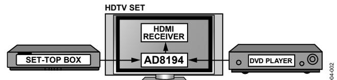
Figure 2. Typical AD8194 Application for HDTV Sets
