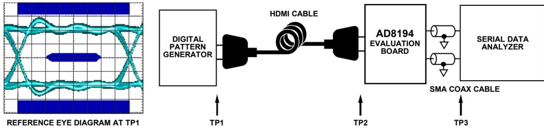
Figure 4. Test Circuit Diagram for Rx Eye Diagrams
