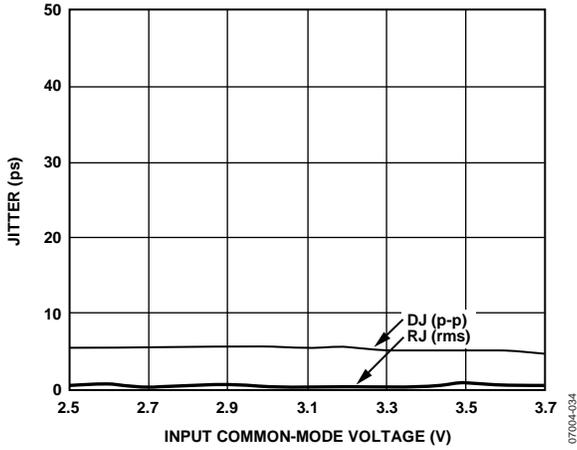
Figure 15. Jitter vs. Input Common-Mode Voltage
