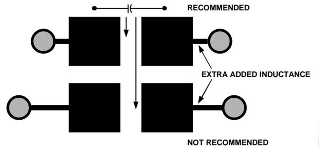
Figure 23. Recommended Pad Outline for Bypass Capacitors
