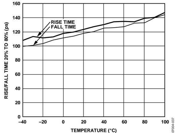
Figure 18. Rise and Fall Time vs. Temperature
