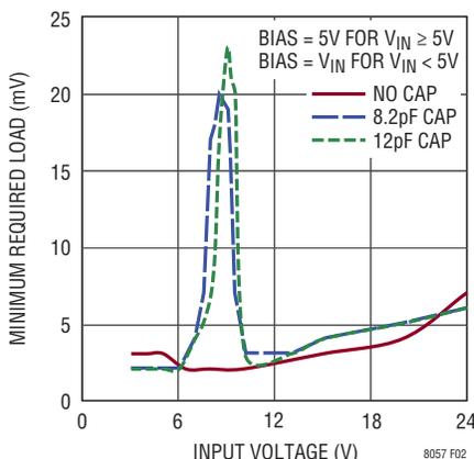
Figure 2. Minimum Required Load vs Input Voltage
