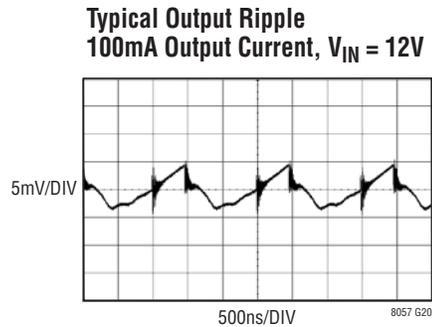
MEASURED ON DC1987 WITH ADDITIONAL  $1\mu\text{F}$  AND BNC ATTACHED TO OUTPUT TERMINALS.  $C_7 = 0.1\mu\text{F}$  USED HP461A 150MHz AMPLIFIER, SET TO 40dB GAIN.
