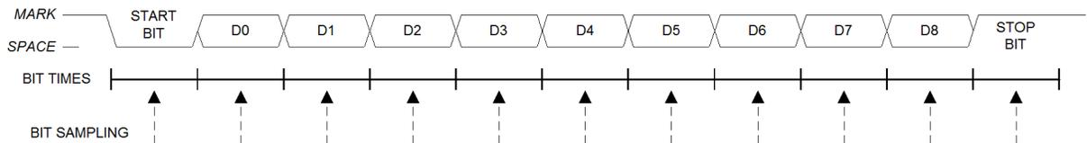
**Figure 21.5. UART0 Modes 2 and 3 Timing Diagram**
