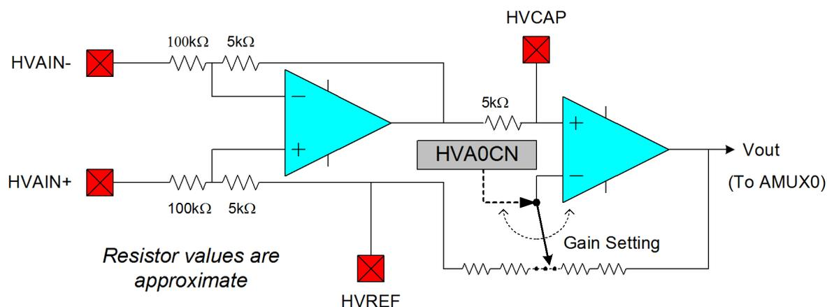
**Figure 5.3. High Voltage Difference Amplifier Functional Diagram**
