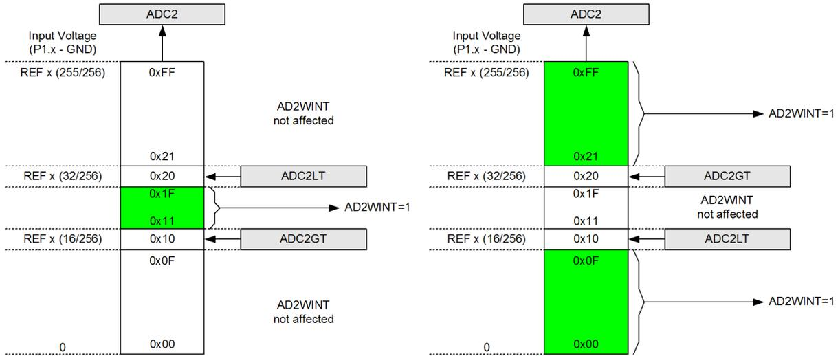
**Figure 7.5. ADC Window Compare Examples, Single-Ended Mode**
