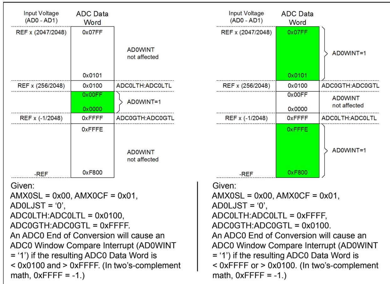
**Figure 5.9. 12-Bit ADC0 Window Interrupt Example:
