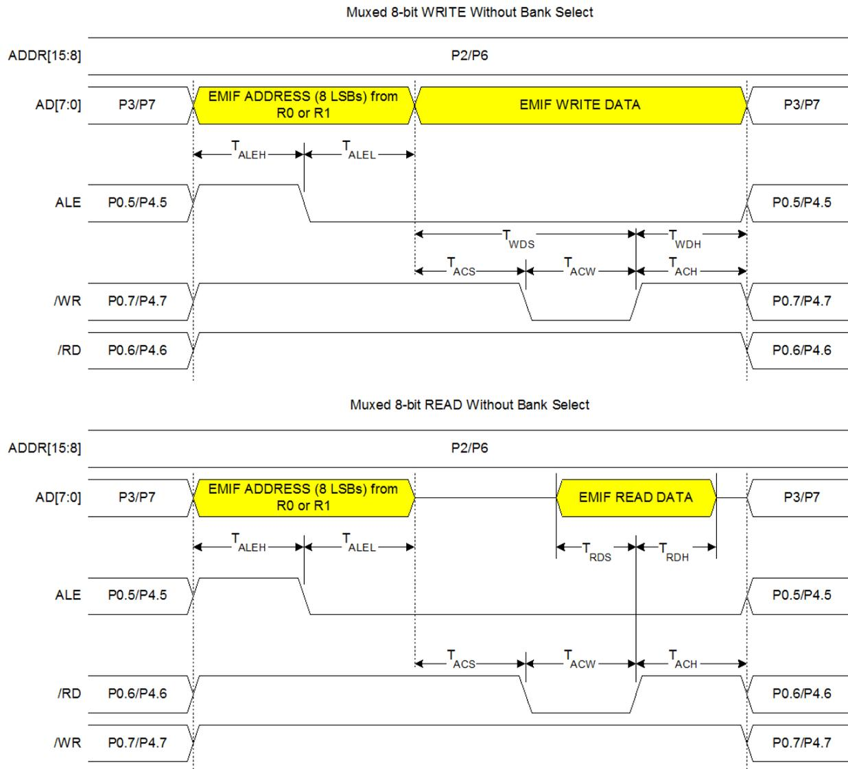
**Figure 16.8. Multiplexed 8-bit MOVX without Bank Select Timing**
