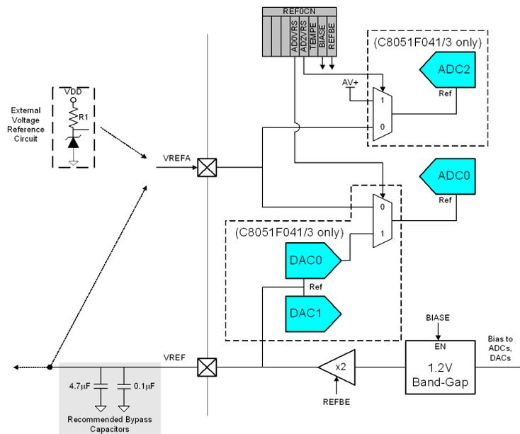
**Figure 10.1. Voltage Reference Functional Block Diagram**
