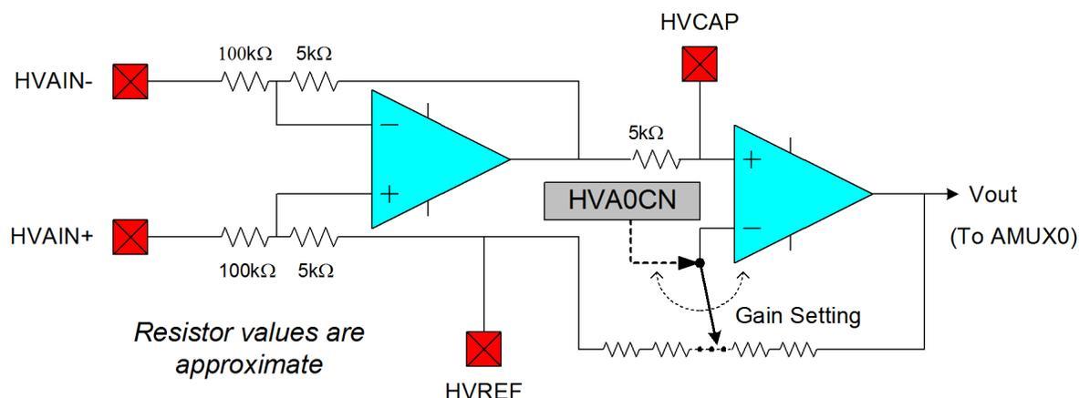
**Figure 6.3. High Voltage Difference Amplifier Functional Diagram**
