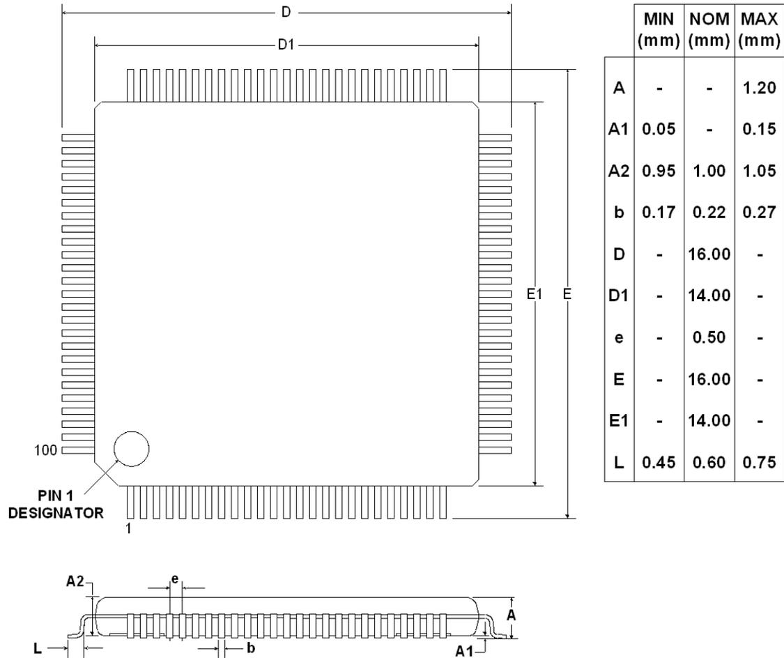
Figure 4.2. TQFP-100 Package Drawing
