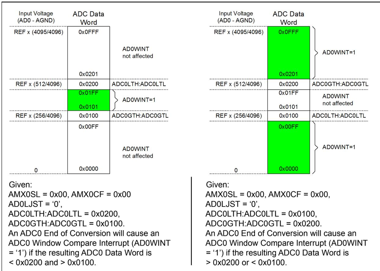
**Figure 5.8. 12-Bit ADC0 Window Interrupt Example:
