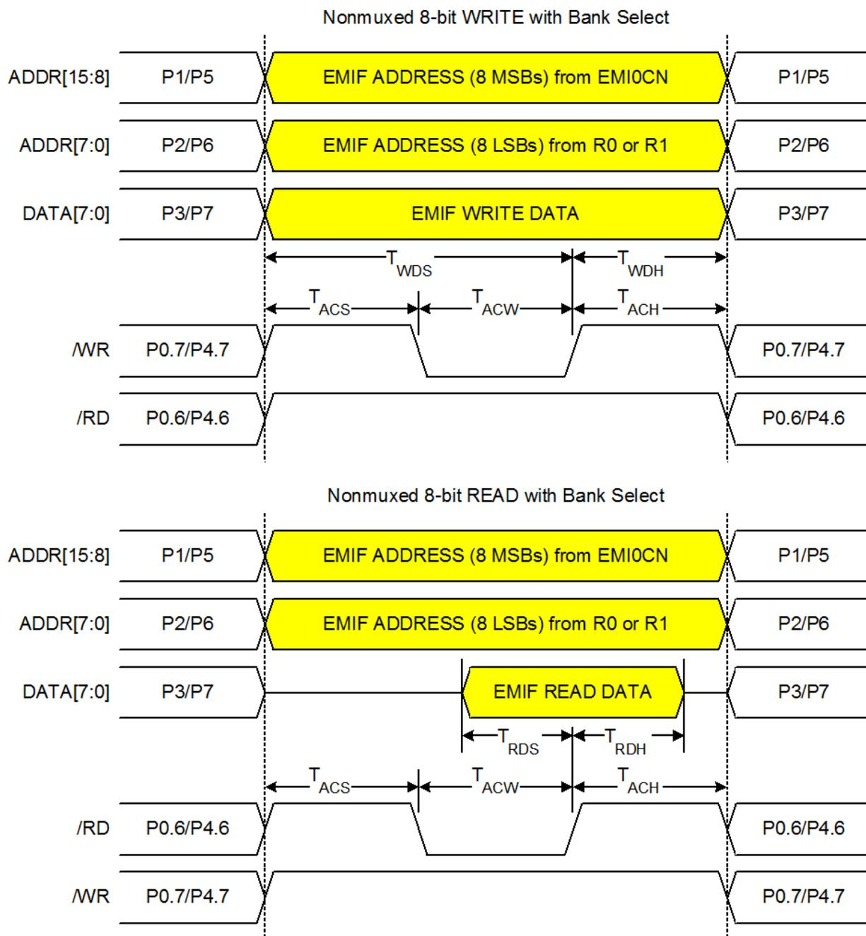
**Figure 16.6. Non-multiplexed 8-bit MOVX with Bank Select Timing**
