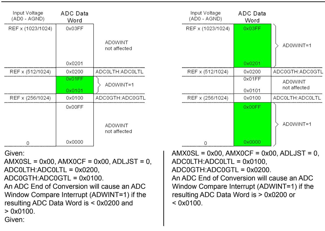
**Figure 6.8. 10-Bit ADC0 Window Interrupt Example:
