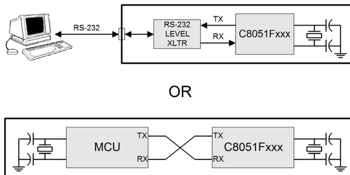
**Figure 21.6. UART0 Modes 1, 2, and 3 Interconnect Diagram**
