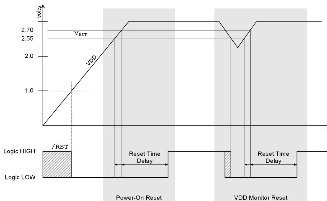
Figure 13.2. Reset Timing
