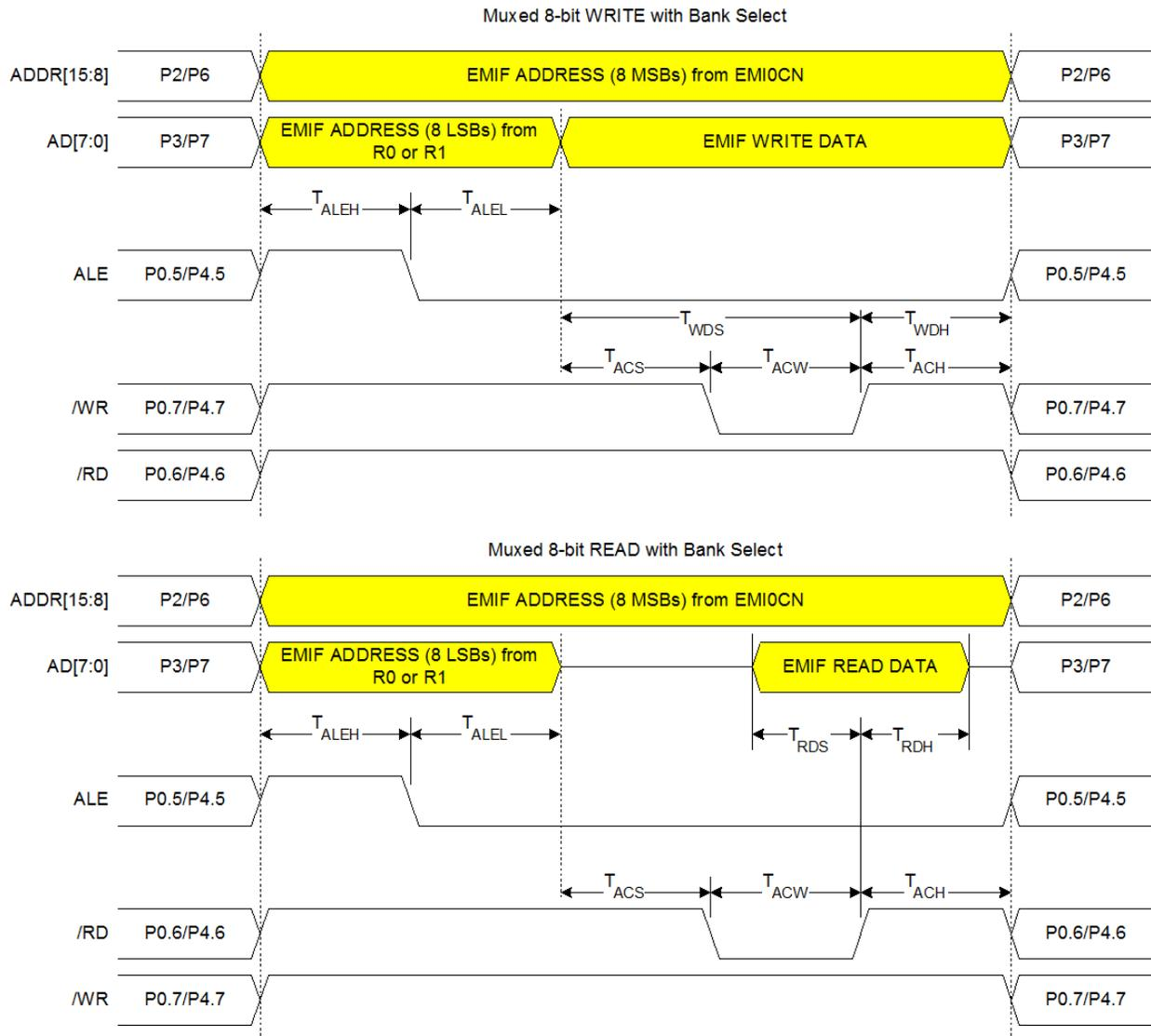
Figure 16.9. Multiplexed 8-bit MOVX with Bank Select Timing
