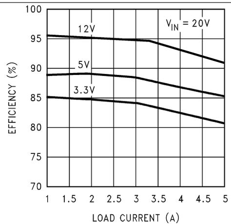
Figure 4. Efficiency vs I<sub>LOAD</sub>
