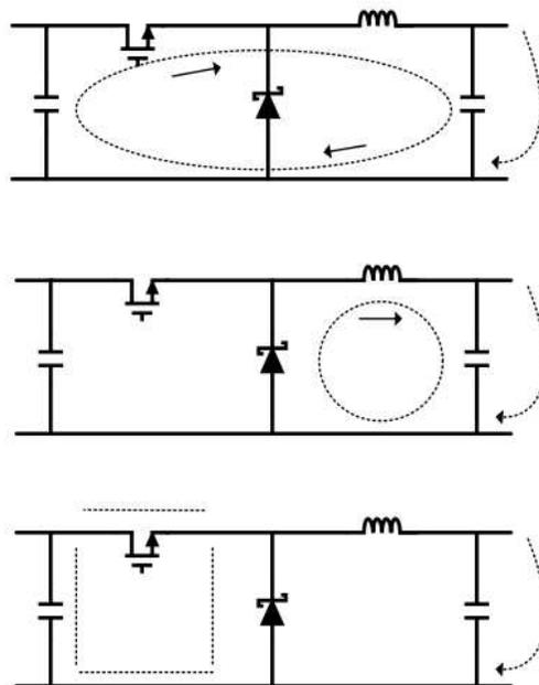
**Figure 23. Typical Current Flow in Buck Regulator**
