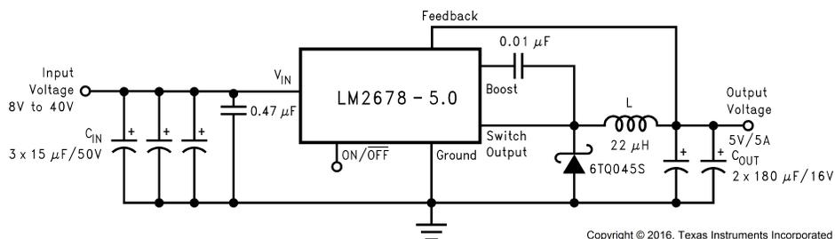
**Figure 16. Typical Application for All Output Voltage Versions**
