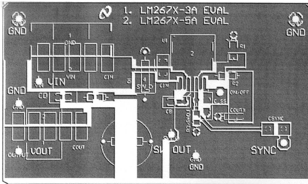
Figure 24. Top Layer Foil Pattern of Printed-Circuit Board
