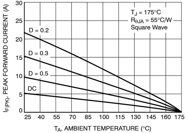
Figure 2. Forward Current Derating of Ambient Temperature
