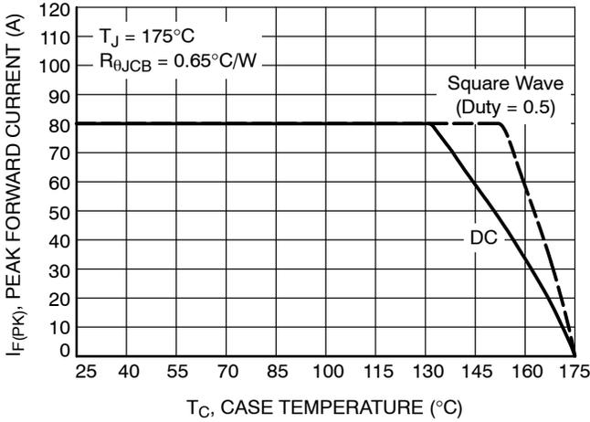
Figure 1. Forward Current Derating of Case Temperature
