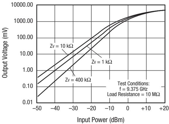
**Figure 3. Typical Zero Bias X-Band Detector Diodes
