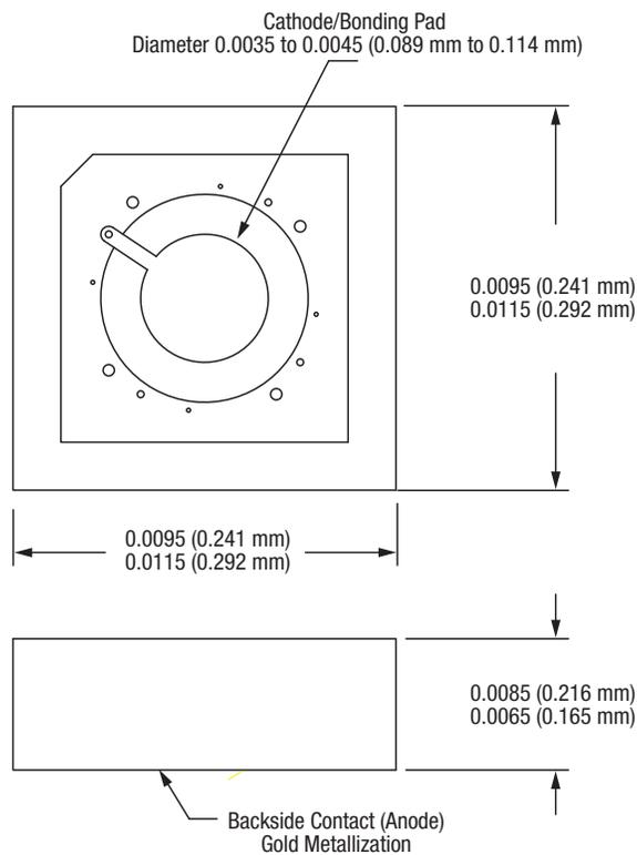
Dimensions are in inches (millimeters shown in parentheses)
