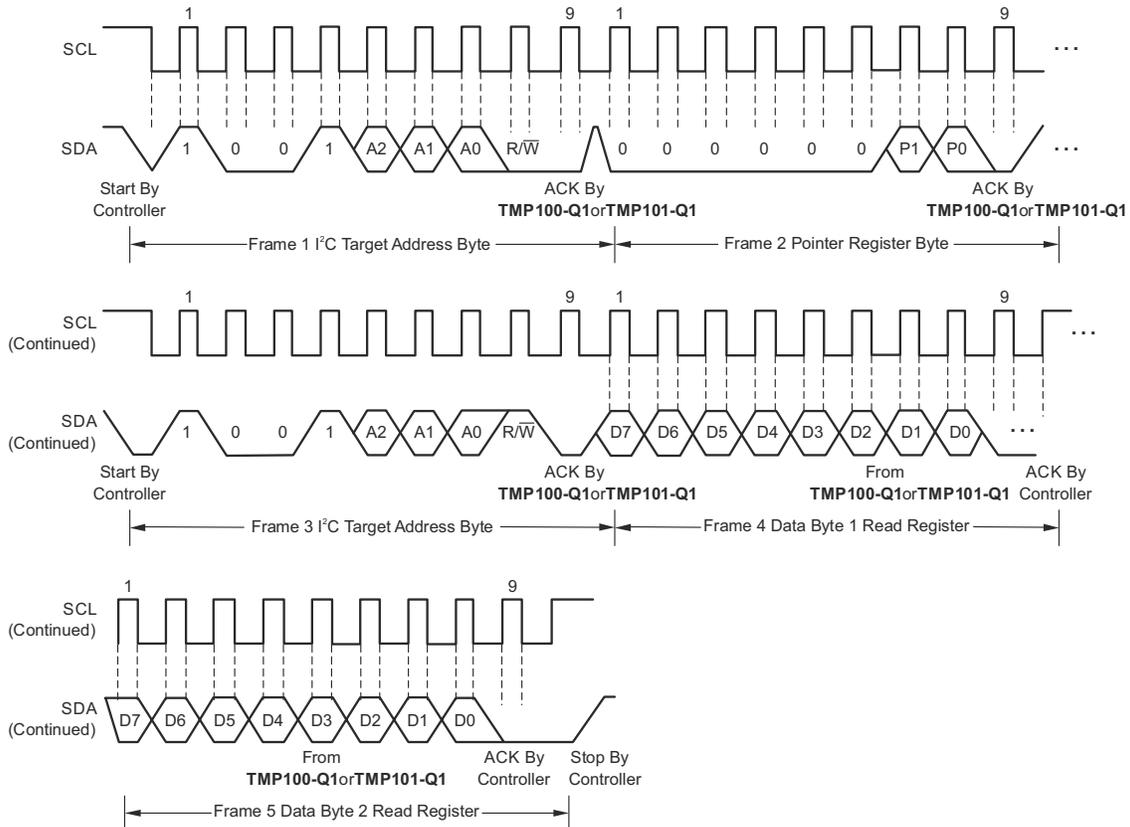
**Figure 7-5. I<sup>2</sup>C Timing Diagram for Read Word Format**
