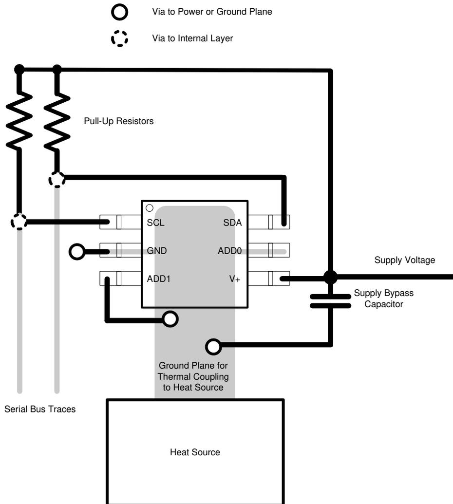
Figure 10-1. TMP100-Q1 Layout Example
