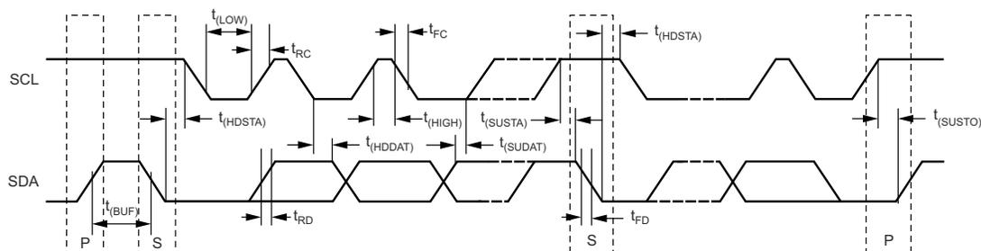
**Figure 7-3. I<sup>2</sup>C Timing Diagram**
