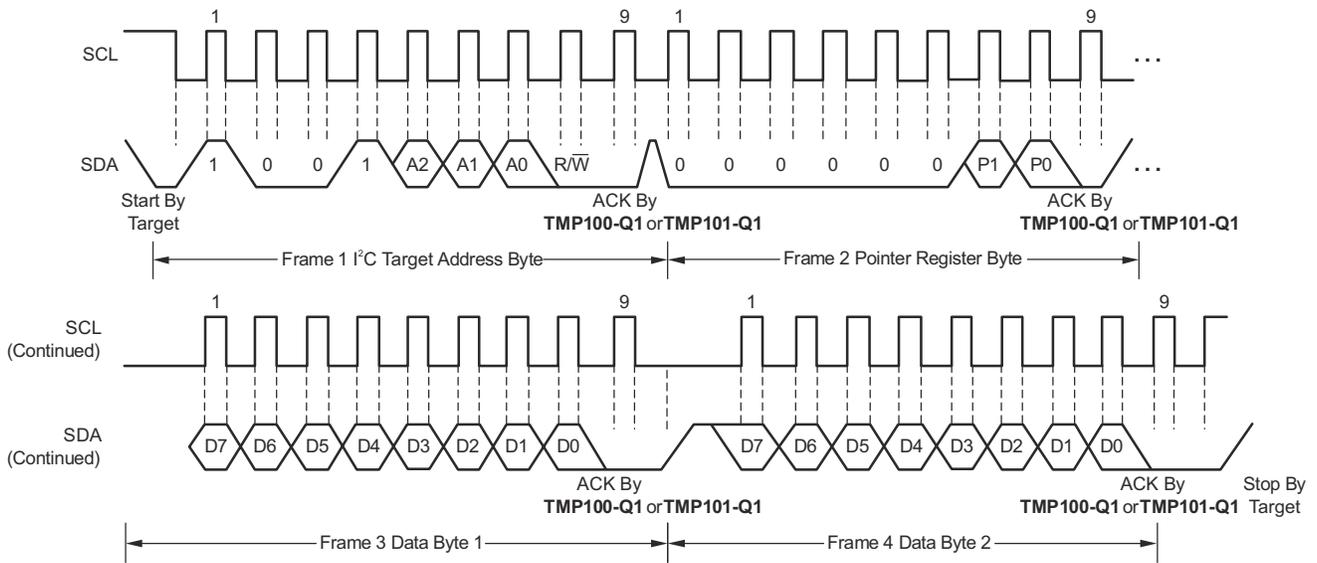
**Figure 7-4. I<sup>2</sup>C Timing Diagram for Write Word Format**
