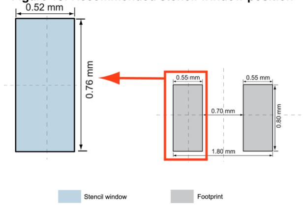
Figure 16: Alternative stencil window position
