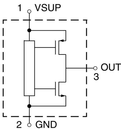
Fig. 4–5: Pin configuration
