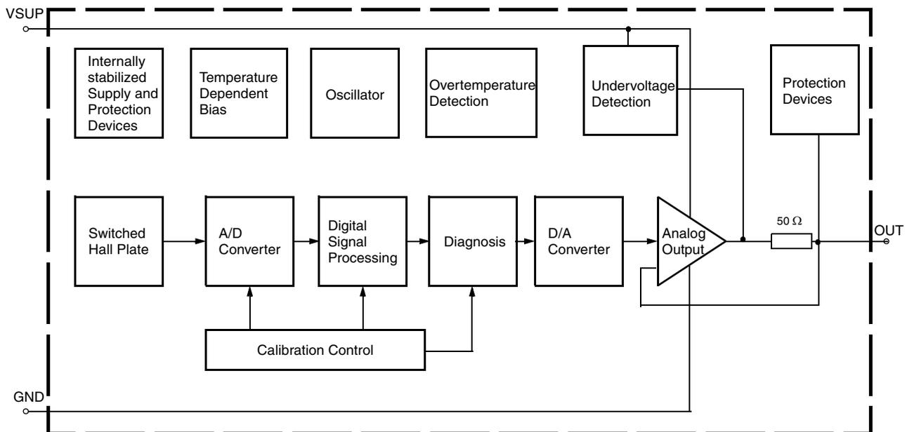
Fig. 3–1: HAL 188x block diagram
