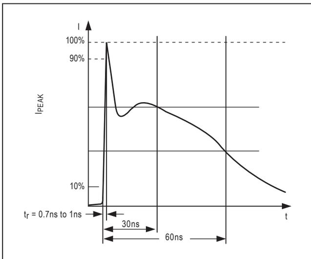
Figure 9b. IEC 61000-4-2 ESD Generator Current Waveform
