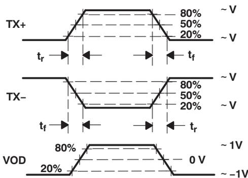
Figure 7. Differential and Common-Mode Output Voltage Definitions
