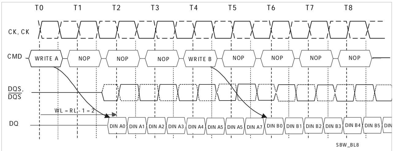
The seamless, non interrupting 8-bit burst write operation is supported by enabling a write command at every  $BL / 2$  number of clocks. This operation is allowed regardless of same or different banks as long as the banks are activated.
