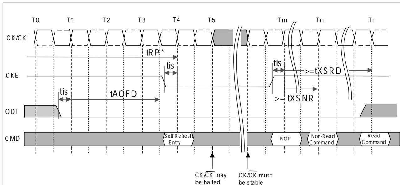
\* = Device must be in the "All banks idle" state to entering Self Refresh mode.
