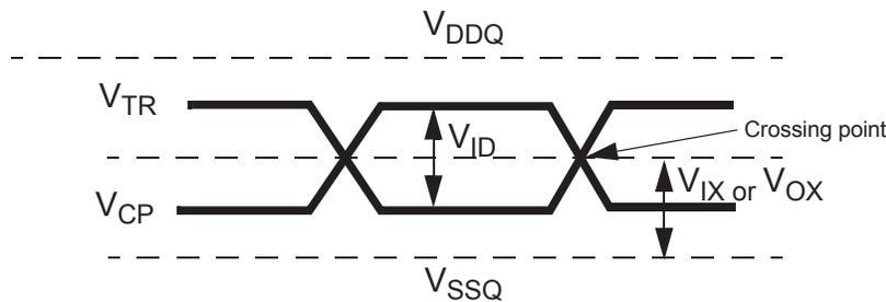
NOTE 1  $V_{ID(AC)}$  specifies the input differential voltage  $|V_{TR} - V_{CP}|$  required for switching, where  $V_{TR}$  is the true input signal (such as  $\overline{CK}$ ,  $\overline{DQS}$ ,  $\overline{LDQS}$  or  $\overline{UDQS}$ ) and  $V_{CP}$  is the complementary input signal (such as  $\overline{CK}$ ,  $\overline{DQS}$ ,  $\overline{LDQS}$  or  $\overline{UDQS}$ ). The minimum value is equal to  $V_{IH(AC)} - V_{IL(AC)}$ .
