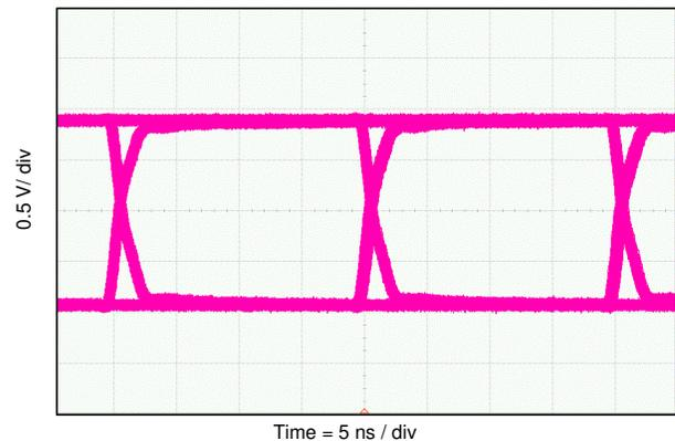
**Figure 9-6. Eye Diagram at 50 Mbps PRBS 2<sup>16</sup> – 1, 1.8 V and 25°C**
