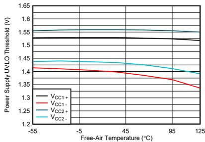
**Figure 6-7. Power Supply Undervoltage Threshold vs Free-Air Temperature**
