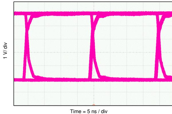
**Figure 9-3. Eye Diagram at 50 Mbps PRBS 2<sup>16</sup> – 1, 5 V and 25°C**
