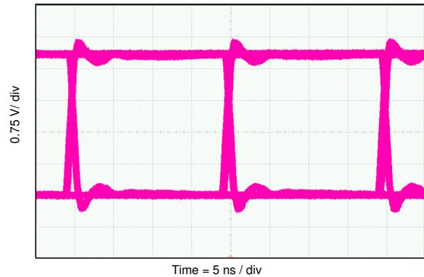
**Figure 9-4. Eye Diagram at 50 Mbps PRBS 2<sup>16</sup> – 1, 3.3 V and 25°C**
