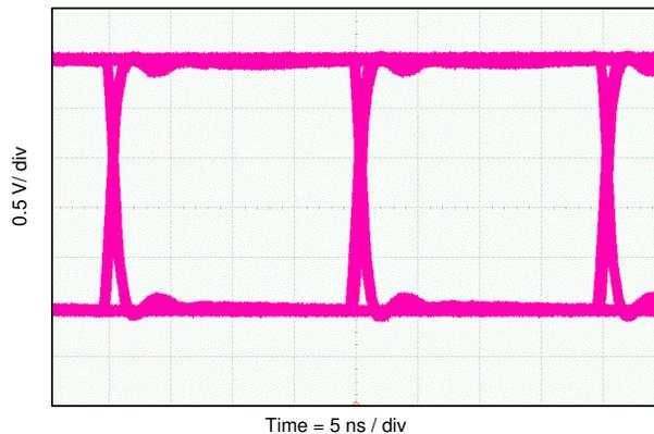
**Figure 9-5. Eye Diagram at 50 Mbps PRBS 2<sup>16</sup> – 1, 2.5 V and 25°C**
