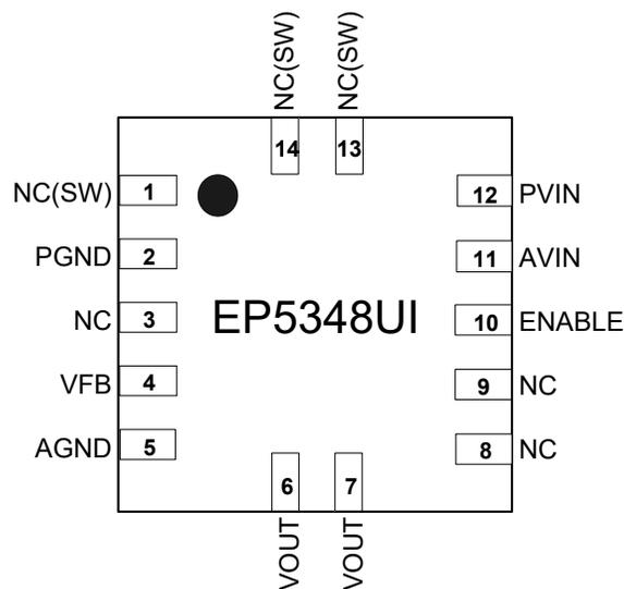
Figure 3: EP5348UI Pin Out Diagram (Top View)
