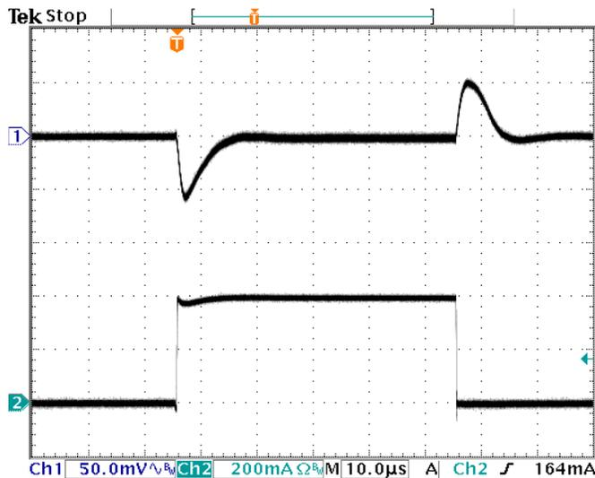
Load Transient:  $V_{IN} = 3.3V$ ,  $V_{OUT} = 1.0V$
