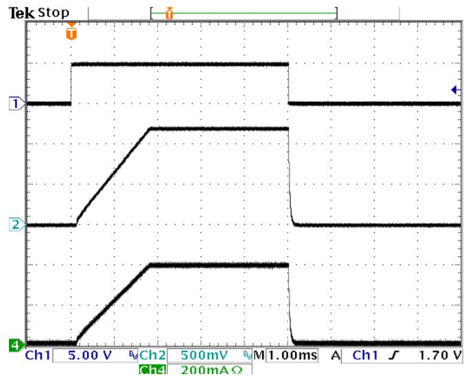
Power Up/Down into  $3\Omega$  load:  $V_{IN}/V_{OUT} = 5.5V/3.3V$ ,
