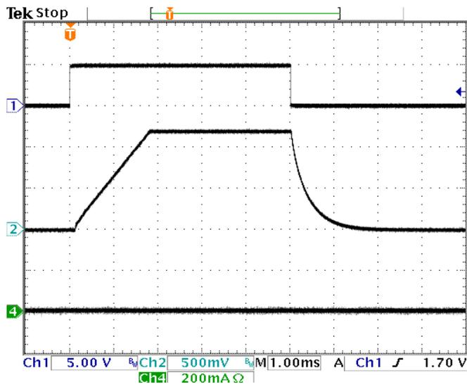
Power Up/Down at No Load:  $V_{IN}/V_{OUT} = 5.0V/1.2V$ ,
