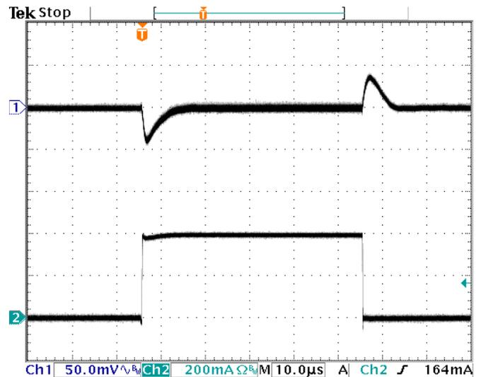
Load Transient:  $V_{IN} = 5V$ ,  $V_{OUT} = 1.0V$
