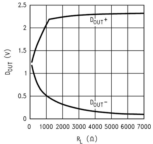
Figure 9. Typical DS90LV031,  $D_O$  vs  $R_L$ ,
