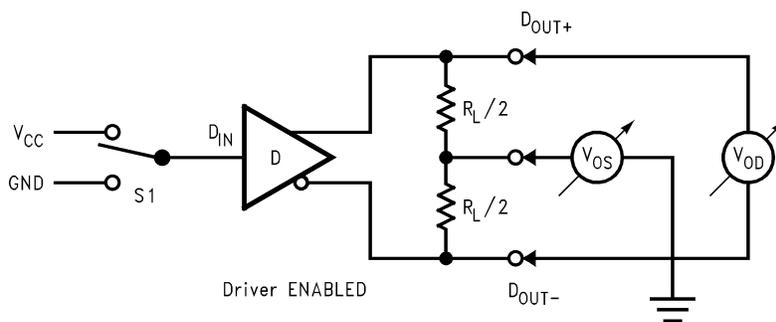
Figure 3. Driver V<sub>OD</sub> and V<sub>OS</sub> Test Circuit
