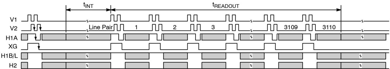
Figure 16. Frame Timing
