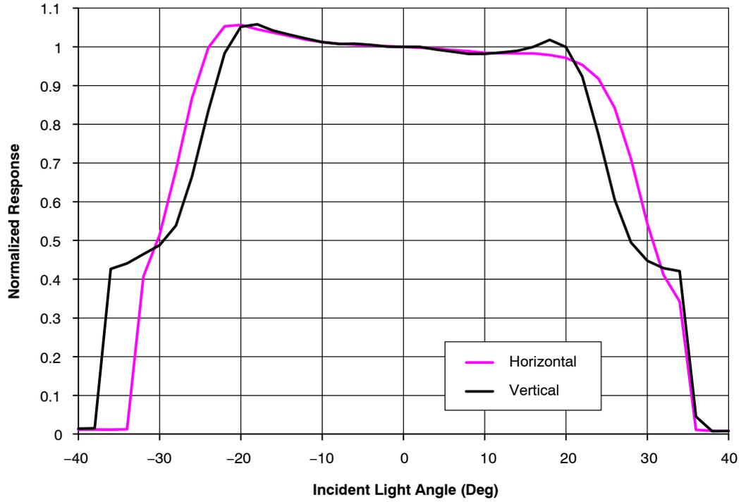
Figure 13. Typical Normalized Angle Response (KAF-50100-ABA Version)
