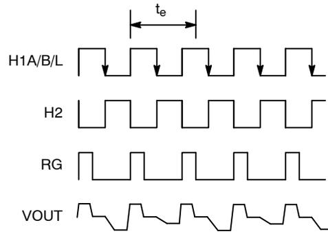
Figure 19. Pixel Timing
