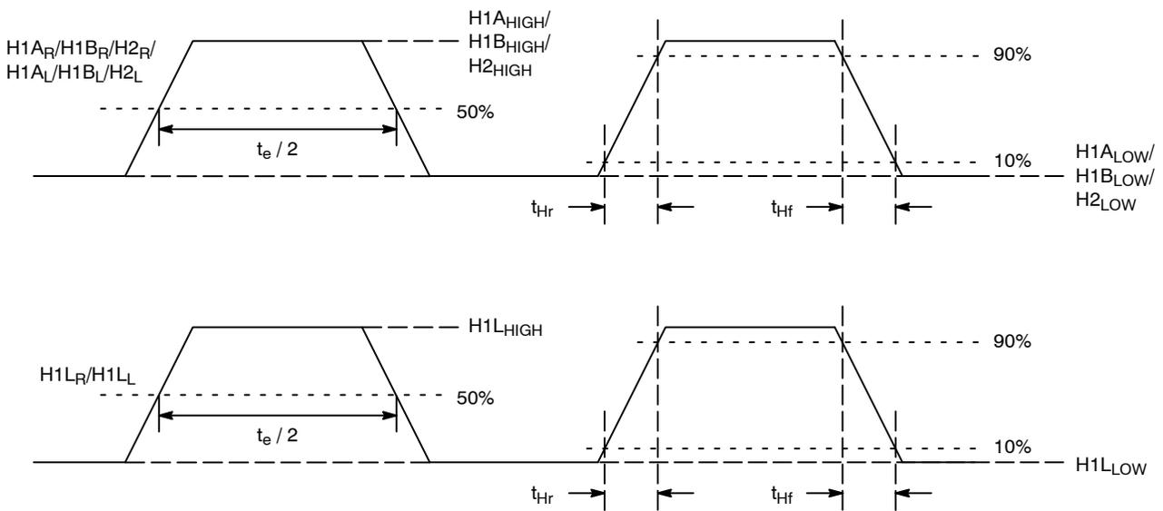
Figure 20. Pixel Timing Detail
