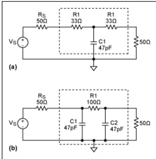
Figure 2a and 2b. EMI filter configurations.
