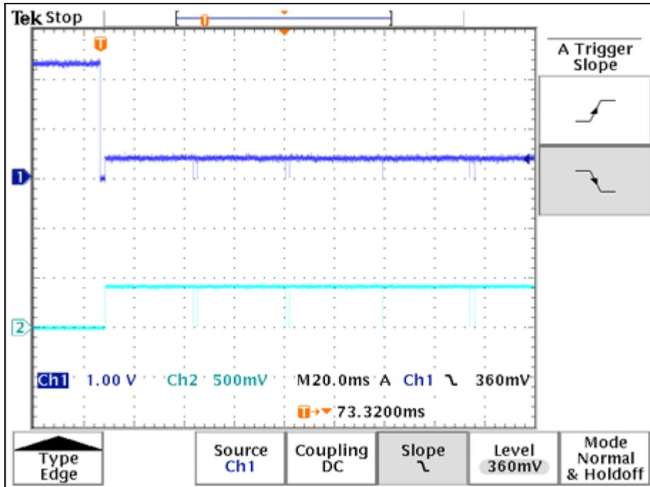
Figure 5. Simulated key-scan PSD levels. Channel 1 shows the column port and channel 2 shows the row port voltages of a MAX7359.
