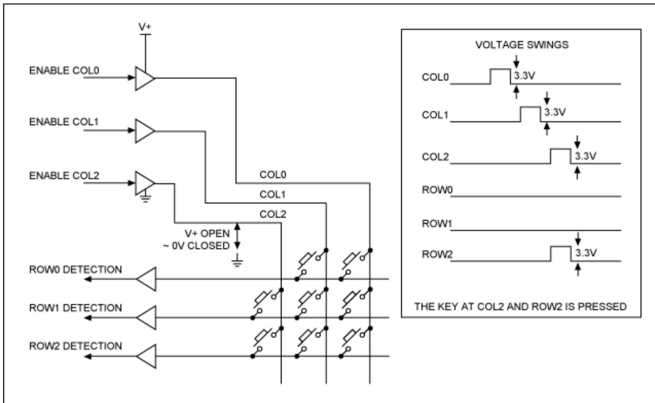
Figure 1. The conventional key scan method.
