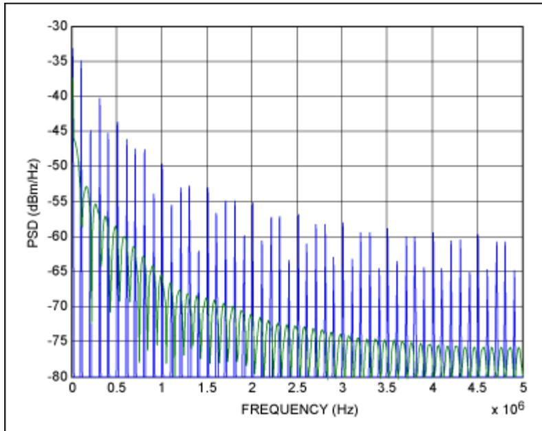
Figure 4. Simulated key scan PSD levels. The blue curve represents the conventional method and the green curve shows Maxim's passive-scan method.
