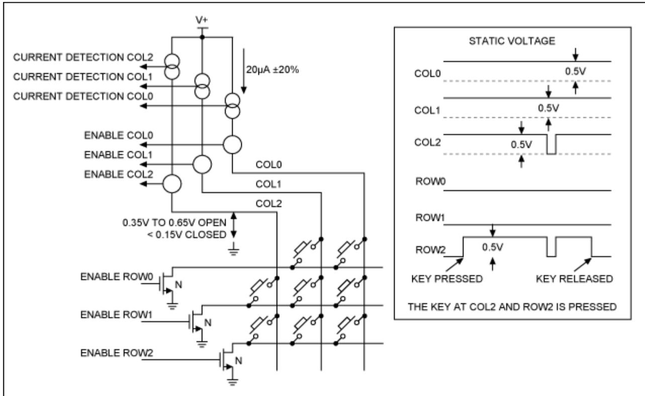
Figure 3. Maxim's low-EMI key-scan method.
