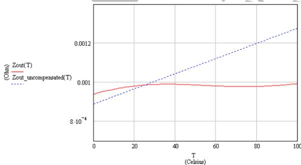
**Figure 21. Uncompensated and Compensated Output Impedance vs. Temperature**
