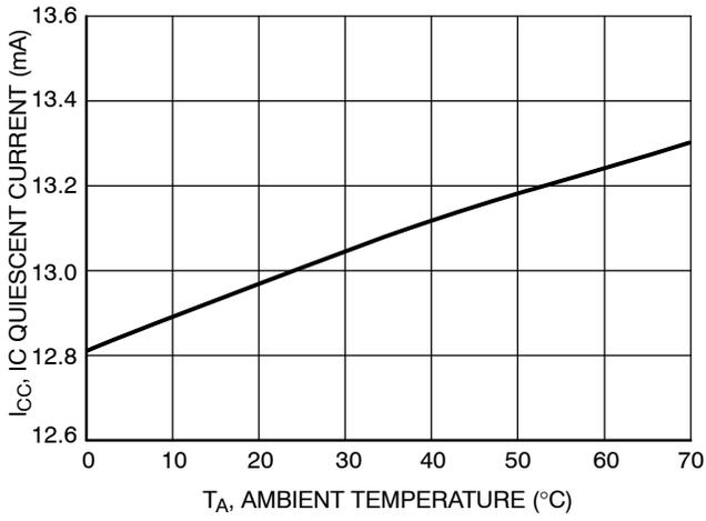
Figure 5. IC Quiescent Current vs. Ambient Temperature
