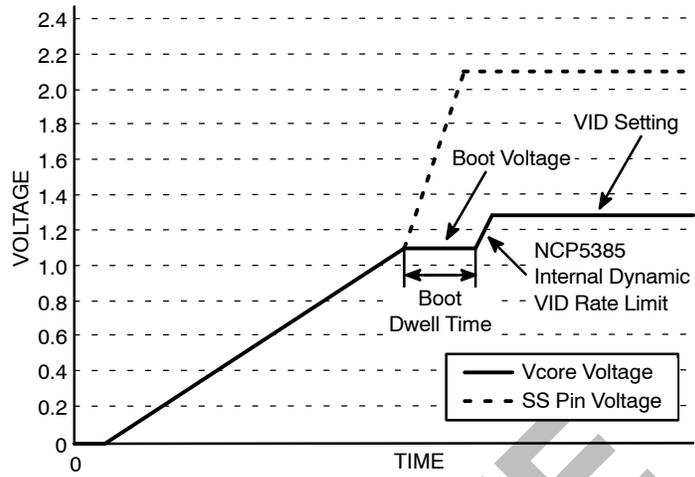
Figure 9. Typical VR11 Soft-Start Sequence to Vcore = 1.3 V
