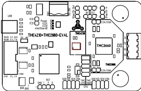
This evaluation board is a development platform for applications based on the TMC4210 and the TMC2660 stepper motor driver IC. The board features USB and CAN interfaces for communication with control software running on a PC. The power MOSFETs of the TMC2660 support drive currents up to 2.8A RMS at 29V.
