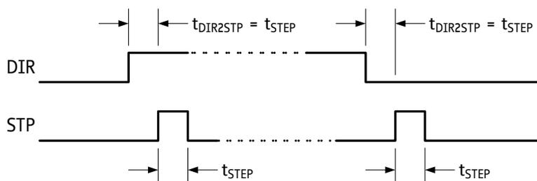
Figure 8.1 Step/Dir timing (*en\_sd* = 1; *step\_half* = 0)
