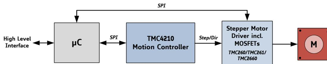
Figure 1.2 Application example using Step/Dir driver interface
