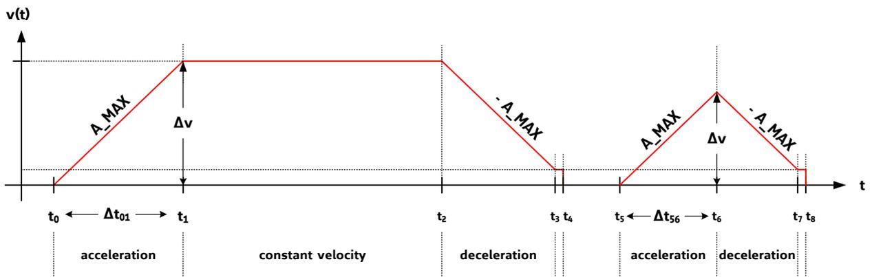
Figure 6.1 Velocity ramp parameters and velocity profiles
