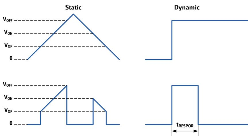
Figure 11.1 Operating principle of the power-on-reset
