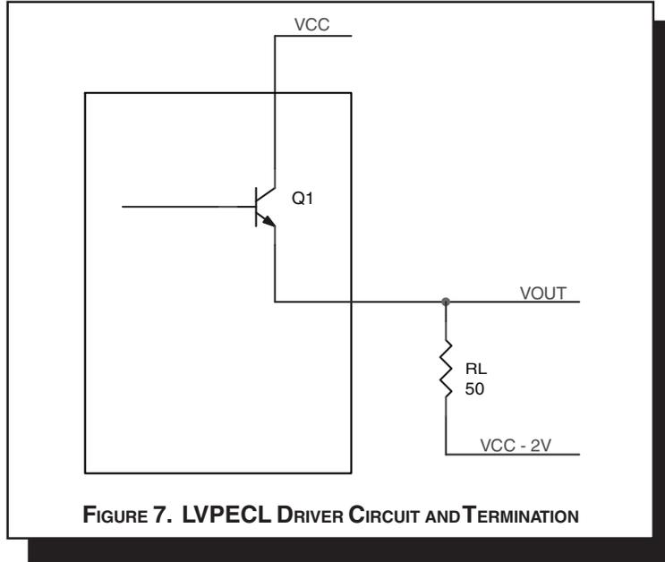
To calculate worst case power dissipation into the load, use the following equations which assume a 50Ω load, and a termination voltage of  $V_{CC} - 2V$ .
