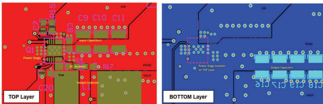
**Figure 14. Recommended PCB Layout (Top Down View)**
