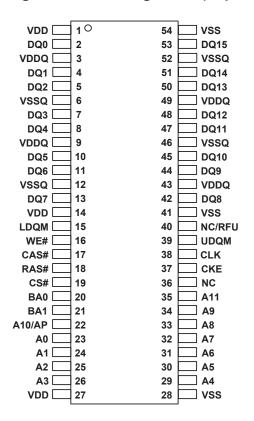
Figure 1.2 Ball Assignment (Top View)
