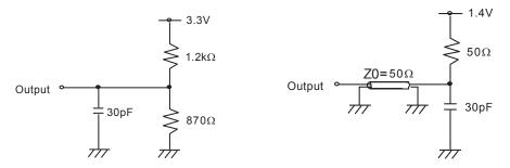
Figure 18.1 LVTTL D.C. Test Load (A)
