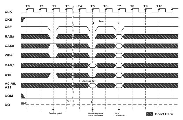
Figure 15. Mode Register Set Cycle
