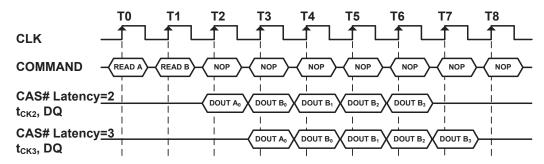
Figure 5. Read Interrupted by a Read (Burst Length = 4, CAS# Latency = 2, 3)
