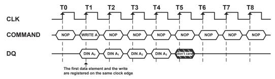
Figure 10. Burst Write Operation (Burst Length = 4)
