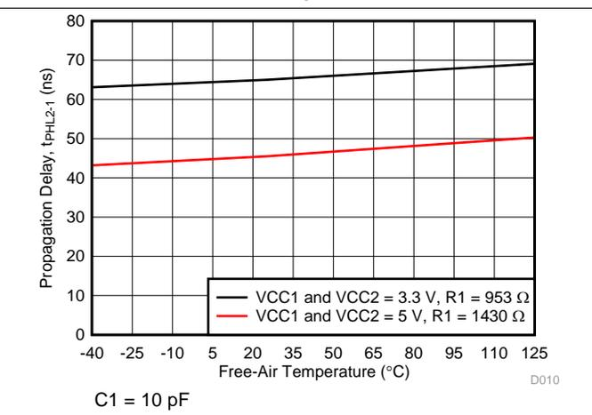
Figure 13.  $t_{PHL2-1}$  Propagation Delay vs Free-Air Temperature
