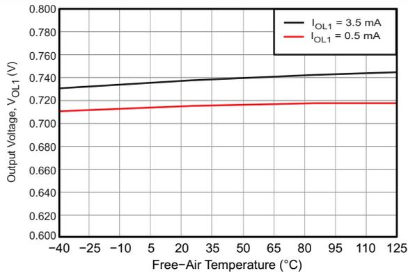
Figure 2. Side 1: Output Low Voltage vs Free-Air Temperature
