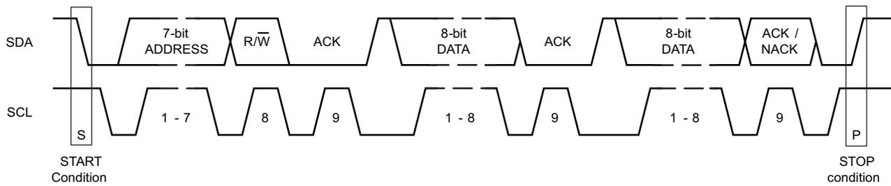
**Figure 28. Timing Diagram of a Complete Data Transfer**
