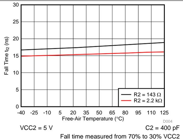
Figure 7. Side 2: Output Fall Time vs Free-Air Temperature
