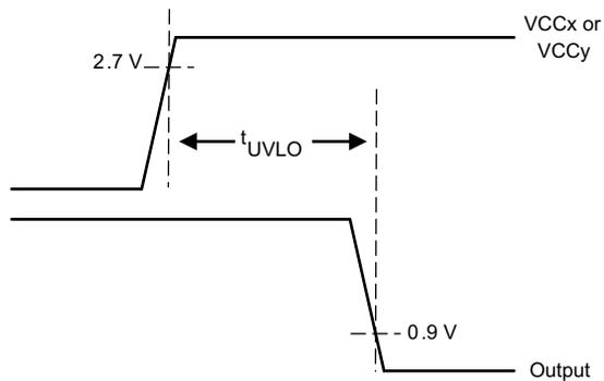
Figure 22.  $t_{UVLO}$  Test Circuit and Timing Diagrams
