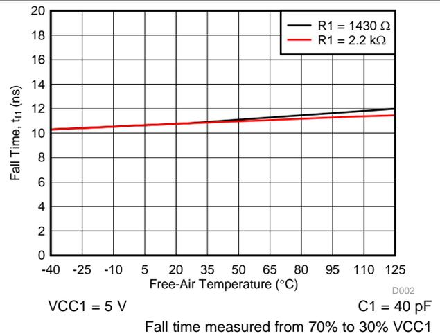
Figure 5. Side 1: Output Fall Time vs Free-air Temperature
