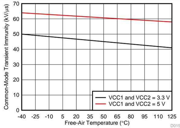
Figure 18. CMTI vs Free-Air Temperature
