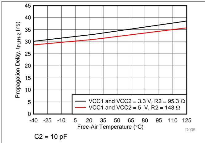
Figure 8.  $t_{PLH1-2}$  Propagation Delay vs Free-Air Temperature
