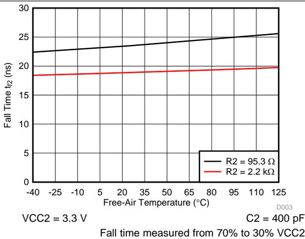
Figure 6. Side 2: Output Fall Time vs Free-Air Temperature
