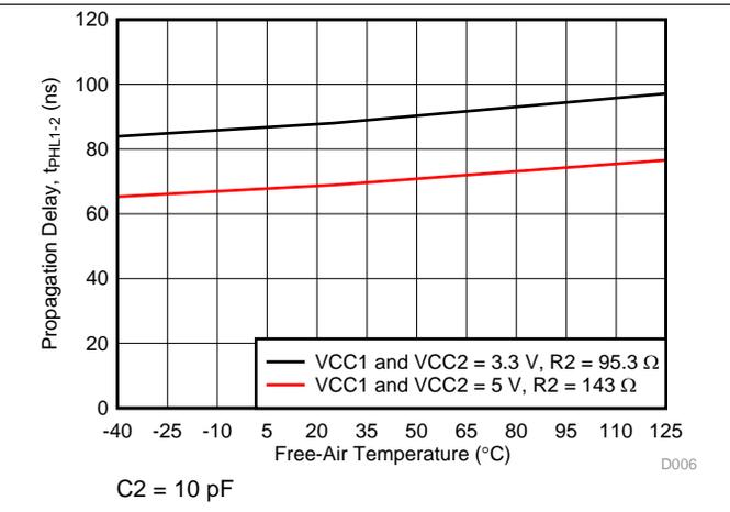
Figure 9.  $t_{PHL1-2}$  Propagation Delay vs Free-Air Temperature
