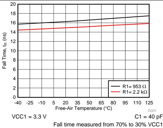
Figure 4. Side 1: Output Fall Time vs Free-Air Temperature
