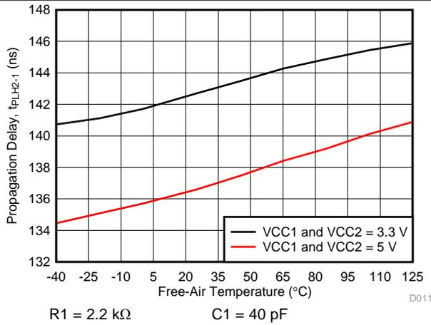
Figure 14.  $t_{PLH2-1}$  Propagation Delay vs Free-Air Temperature
