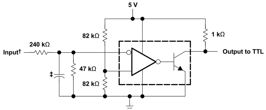
† Resistor values shown are for a 0- to 30-V logic swing and a 15-V threshold.
