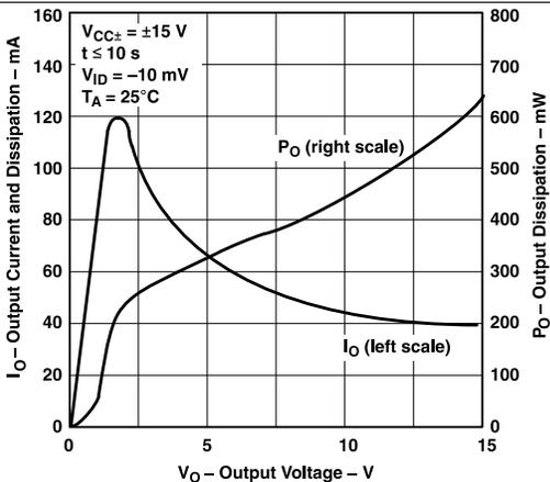
Figure 5. Output Current and Dissipation vs Output Voltage
