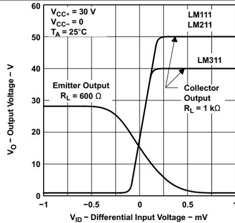
Figure 8. Voltage Transfer Characteristics and Test Circuits
