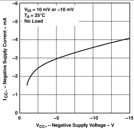
Figure 7. Negative Supply Current vs Negative Supply Voltage
