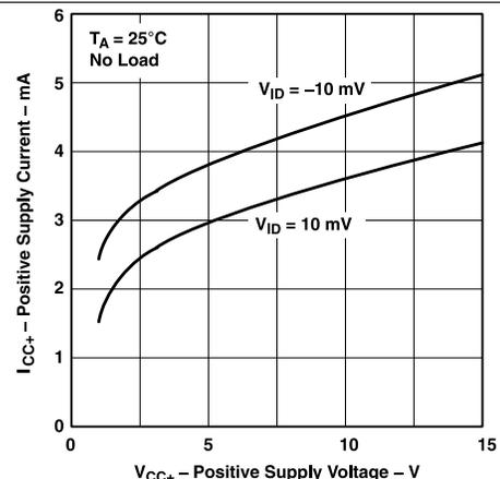
Figure 6. Positive Supply Current vs Positive Supply Voltage
