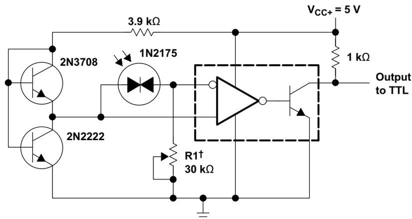
† R1 sets the comparison level. At comparison, the photodiode has less than 5 mV across it, decreasing dark current by an order of magnitude.
