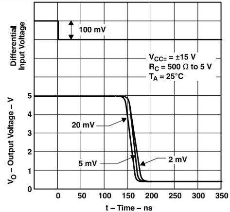
Figure 4. Output Response for Various Input Overdrives
