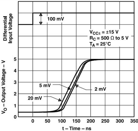
Figure 3. Output Response for Various Input Overdrives
