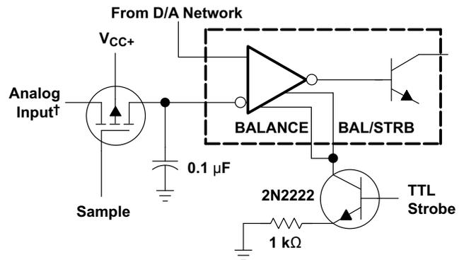
† Typical input current is 50 pA with inputs strobed off.
