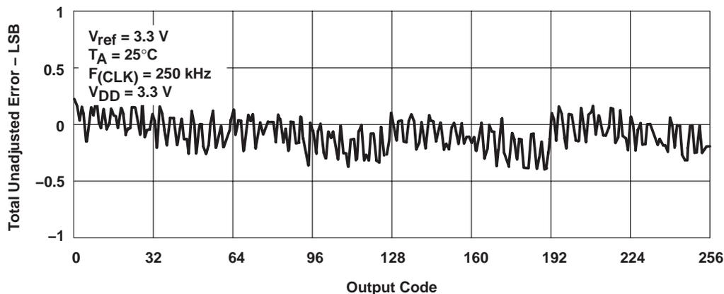
Figure 13. Total Unadjusted Error With Output Code
