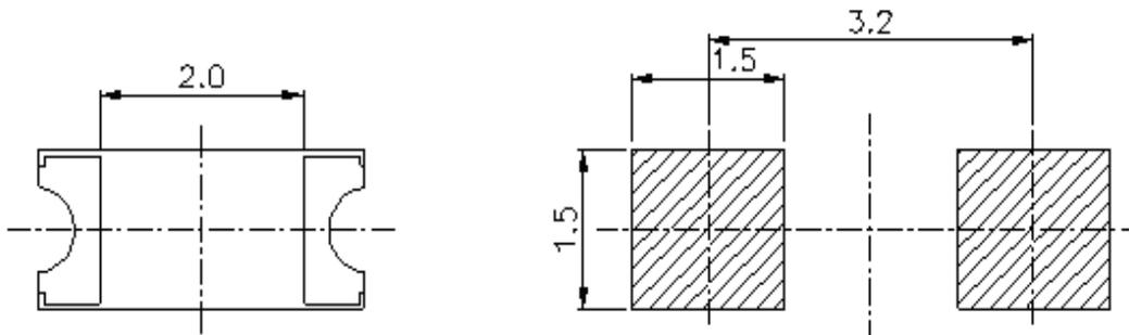
**Note:** The tolerances unless mentioned is  $\pm 0.1\text{mm}$ , Unit = mm
