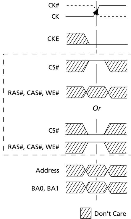
Figure 51: Power-Down Mode (Active or Precharge)
