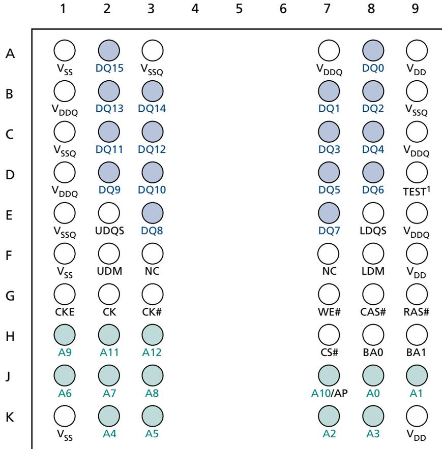
Note: 1. D9 is a test pin that must be tied to V<sub>SS</sub> or V<sub>SSQ</sub> in normal operations.
