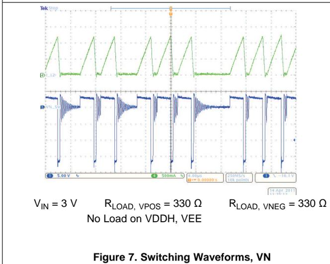
**Figure 7. Switching Waveforms, VN**
