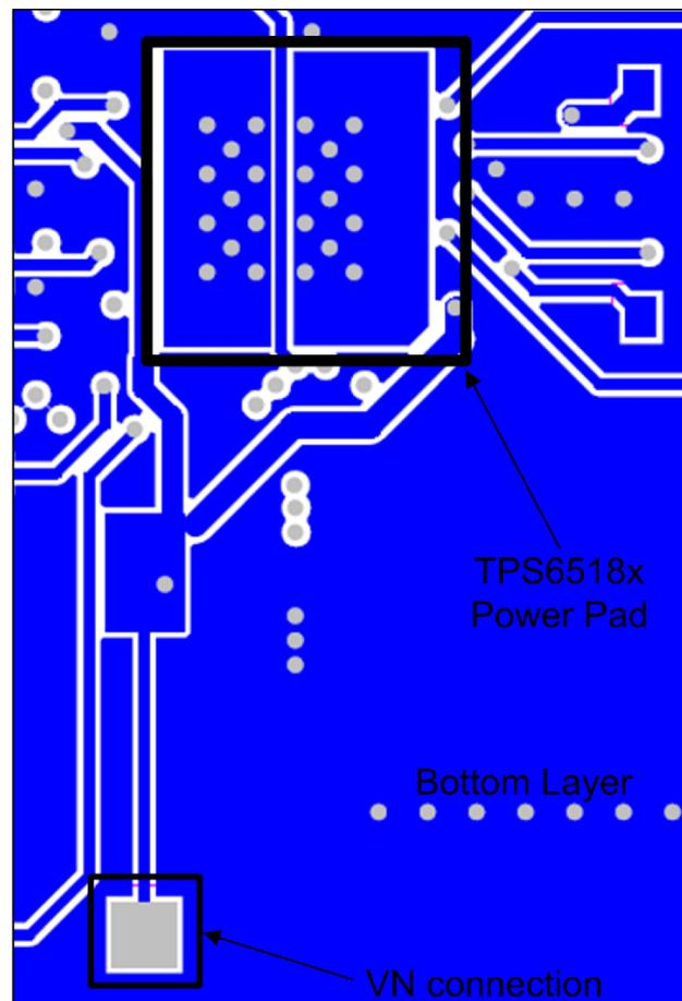
**Figure 33. Layout Diagram**
