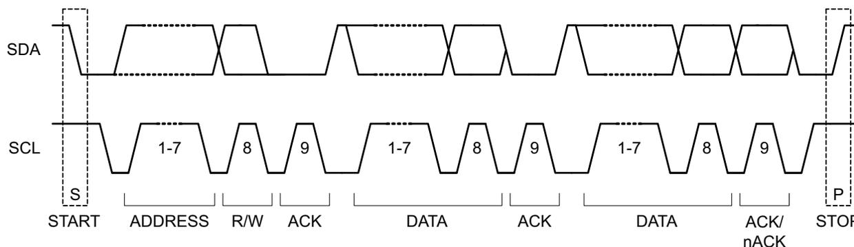
Figure 27. I<sup>2</sup>C Start/Stop/Acknowledge Protocol
