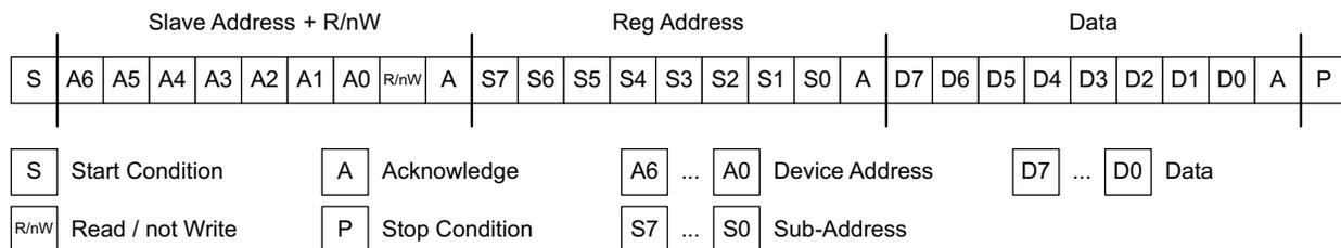
Figure 25. Subaddress in I<sup>2</sup>C Transmission
