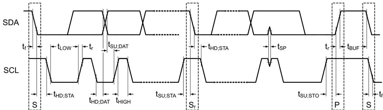
**Figure 1. I<sup>2</sup>C Data Transmission Timing**
