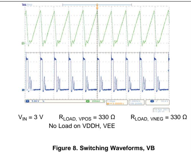
**Figure 8. Switching Waveforms, VB**
