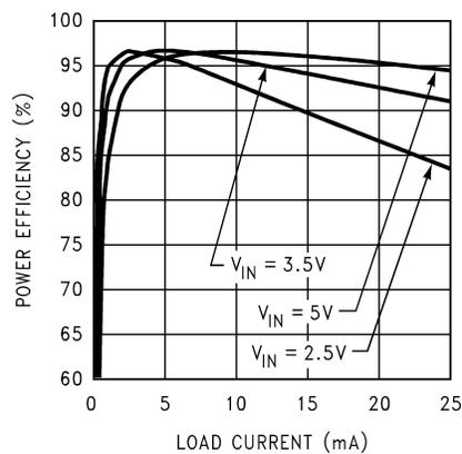
Figure 16. Efficiency vs Load Current
