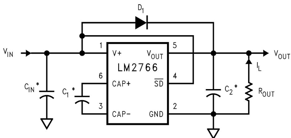
\*  $C_{IN}$ ,  $C_1$ , and  $C_2$  are  $1.0\ \mu\text{F}$  OS-CON capacitors.
