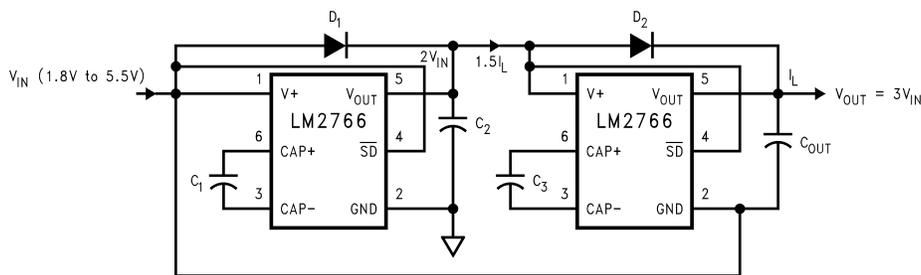
**Figure 14. Increasing Output Voltage By Cascading Devices**
