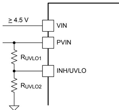
Figure 44. Adjustable PVIN Undervoltage Lockout, (VIN  $\geq 4.5$  V)
