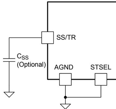
**Figure 32. Slow-Start Capacitor (C<sub>SS</sub>) and STSEL Connection**
