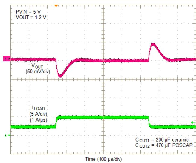
Figure 20. PVIN = 5 V, VOUT = 1.2 V, 2.5 A Load Step
