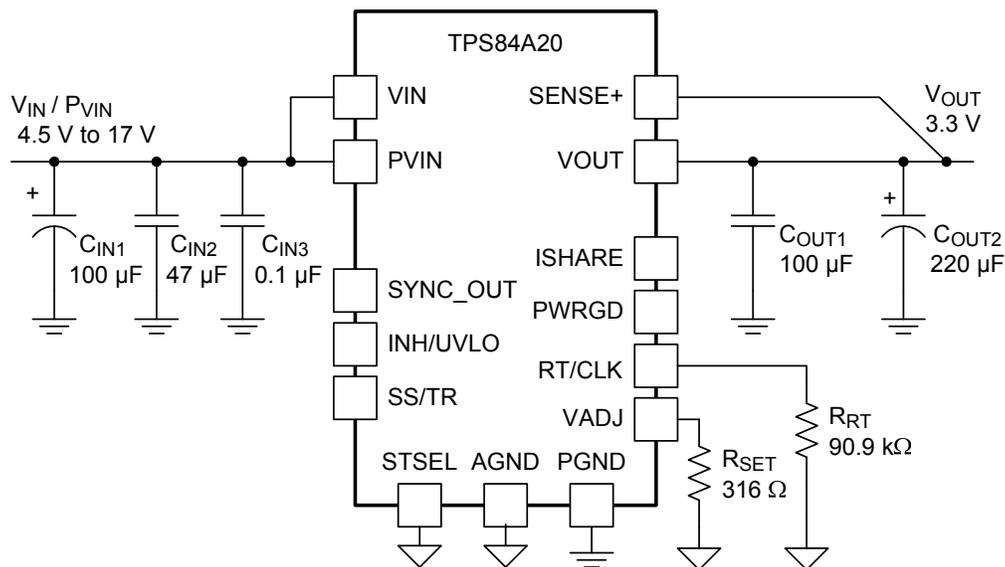
Figure 24. Typical Schematic
