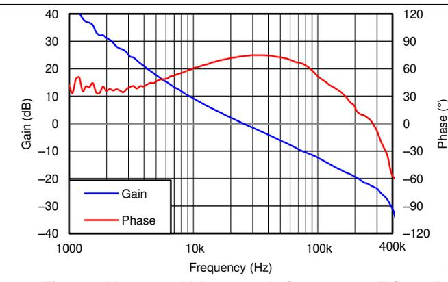
Figure 4. V<sub>OUT</sub> = 1.8 V, I<sub>OUT</sub> = 10 A, C<sub>OUT1</sub> = 200 μF Ceramic, f<sub>sw</sub> = 500 kHz
