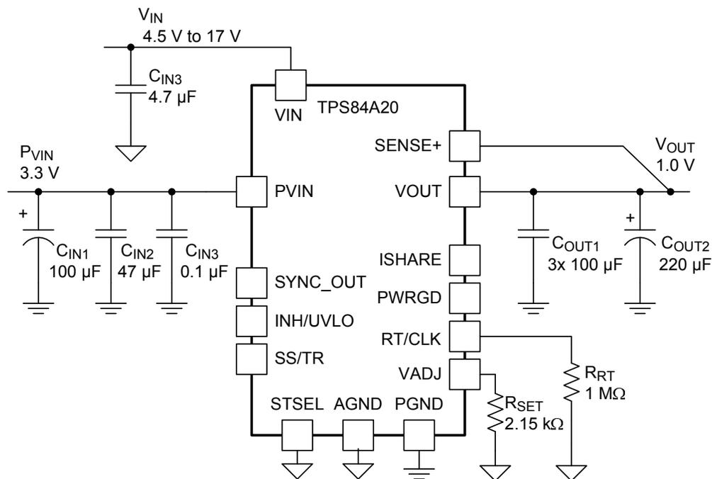
Figure 25. Typical Schematic
