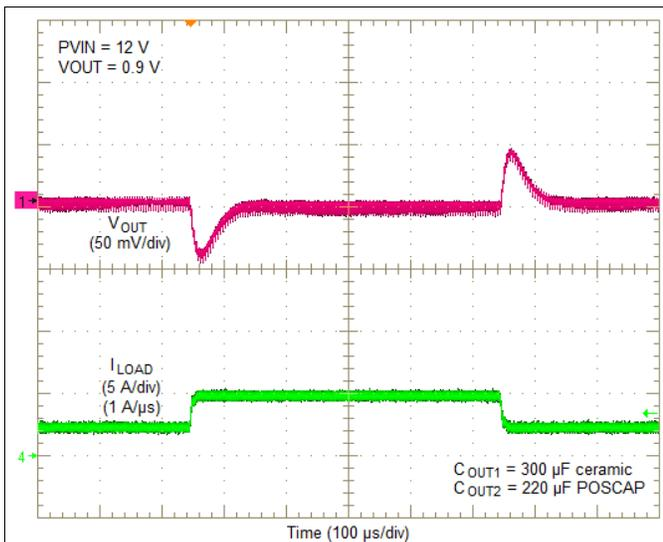
Figure 17. PVIN = 12 V, VOUT = 0.9 V, 2.5 A Load Step
