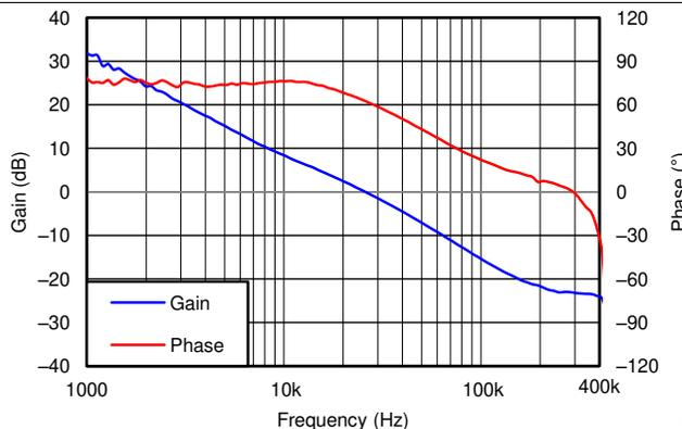
Figure 15. V<sub>OUT</sub> = 1.8 V, I<sub>OUT</sub> = 10 A, C<sub>OUT1</sub> = 200 μF Ceramic, f<sub>sw</sub> = 500 kHz
