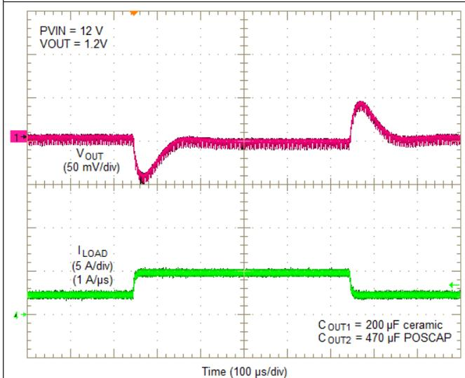
Figure 19. PVIN = 12 V, VOUT = 1.2 V, 2.5 A Load Step
