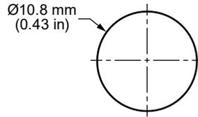
Figure 2. ANT-DB1-WRT-MON Series Antenna Recommended Enclosure Mounting Dimensions
