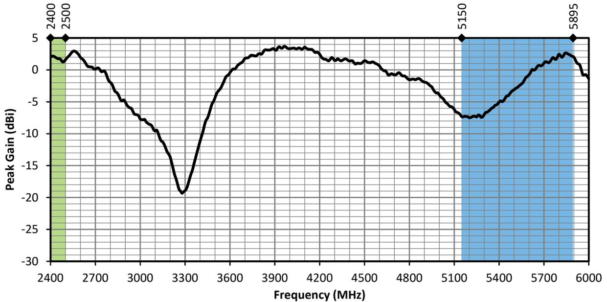
Figure 6. ANT-DB1-WRT-MON Peak Gain, with Frequency Band Highlights
