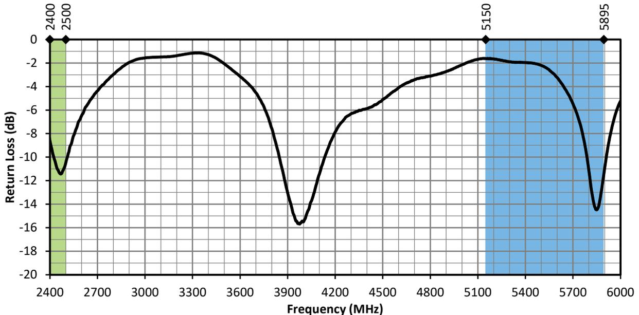
Figure 5. ANT-DB1-WRT-MON Return Loss, with Frequency Band Highlights
