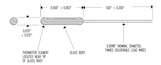
RESISTANCE @  $+25^{\circ}$ C = 5,000  $\Omega$  ± 5% RESISTANCE/TEMPERATURE CURVE = "F" BETA " $\beta$ " (+25 TO +85°C) = 3,499°K NOMINAL TEMPERATURE COEFFICIENT @  $+25^{\circ}$ C = -3.86%/°C NOMINAL TEMPERATURE RATING = -50 TO  $+300^{\circ}$ C
