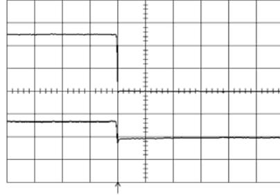
Shut-down enabled by disconnecting  $V_i$  at:
