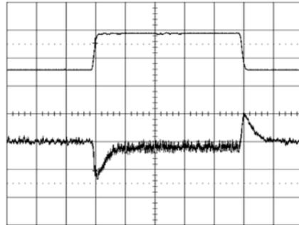
Output voltage response to load current step-
