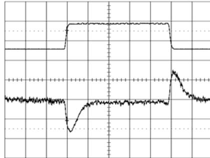
Output voltage response to load current step-
