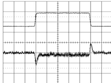
Output voltage response to load current step-
