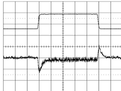
Output voltage response to load current step-
