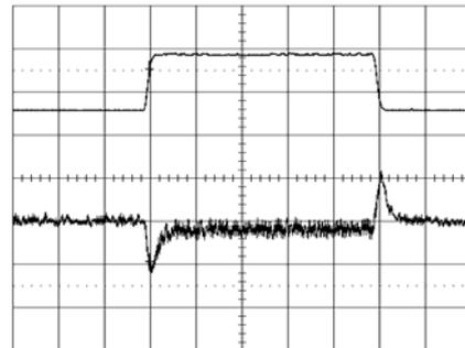
Output voltage response to load current step-
