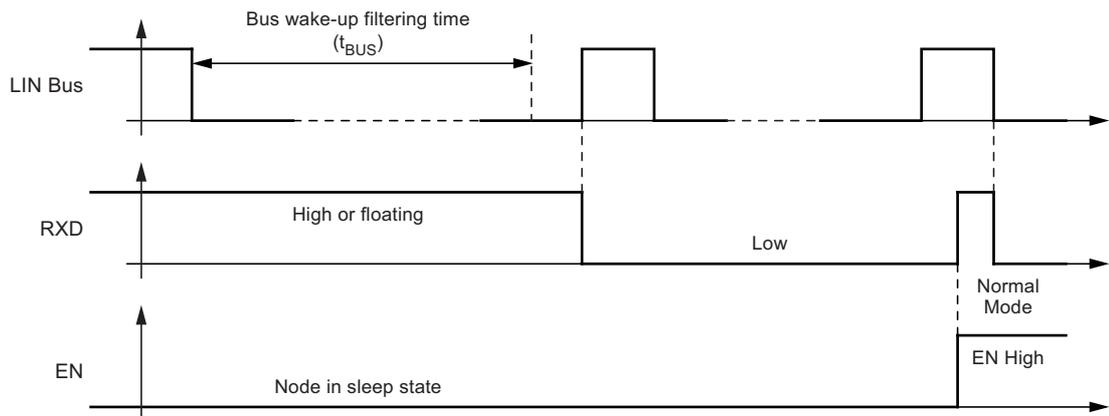
In Sleep mode the device has a very low current consumption even during short-circuits or floating conditions on the bus. A floating bus can arise if the master pull-up resistor is missing, e.g., it is switched off when the LIN master is in sleep mode or even if the power supply of the master node is switched off.
