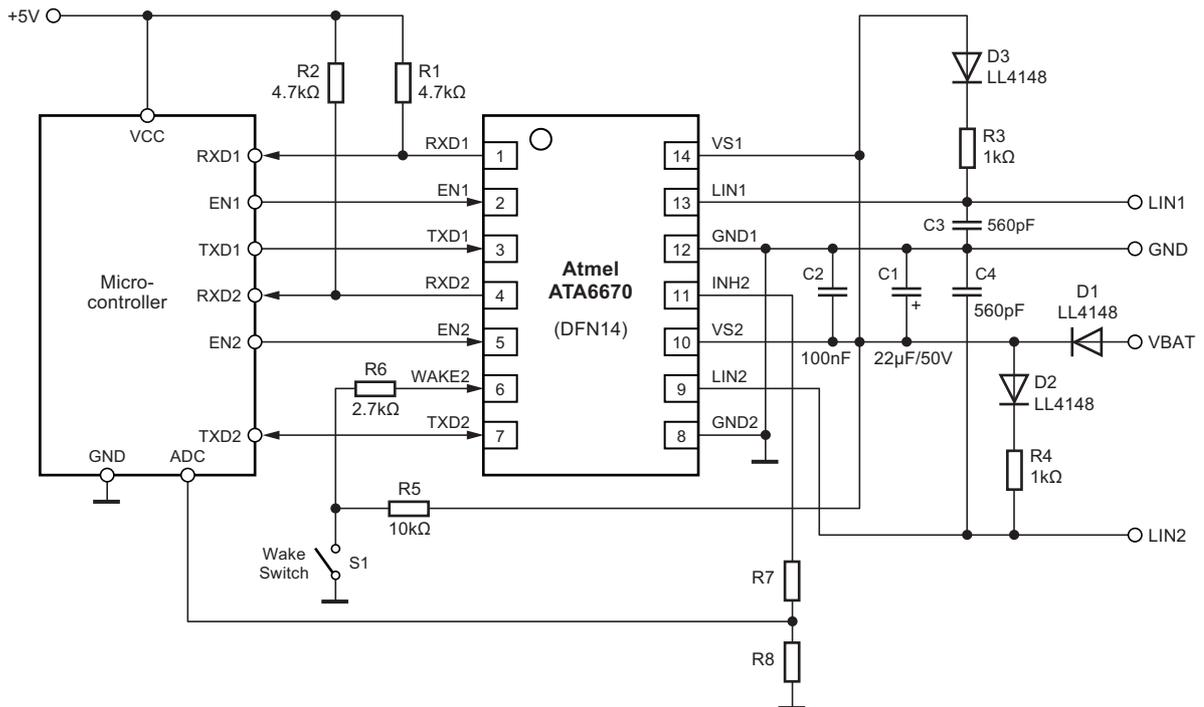
**Figure 5-3. Application with Minimum External Devices: INH2 Output and WAKE2 Input Not Used**
