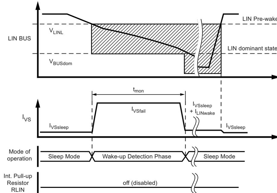
If the Atmel® ATA6670 is in sleep mode and the voltage level at the LIN is in dominant state ( $V_{LIN} < V_{BUSdom}$ ) for a period of time exceeding  $t_{mon}$  (during a short circuit at LIN, for example), the IC switches back to sleep mode. The VS current consumption then consists of  $I_{VSsleep}$  plus  $I_{LINWAKE}$ . After a positive edge at pin LIN the IC switches directly to fail-safe mode (see Figure 2-4).
