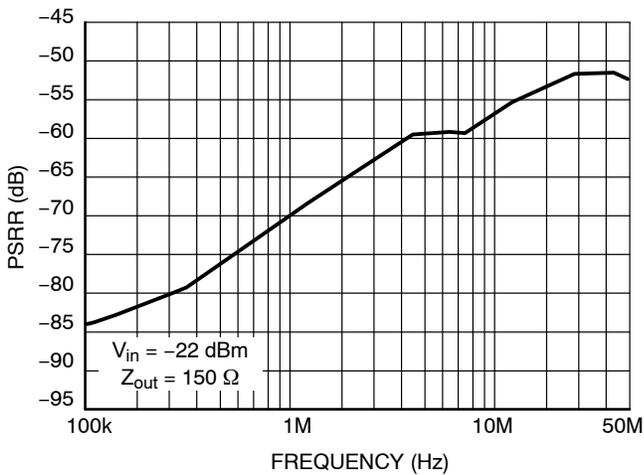
Figure 7. PSRR vs Frequency (No Bypass Capacitor)
