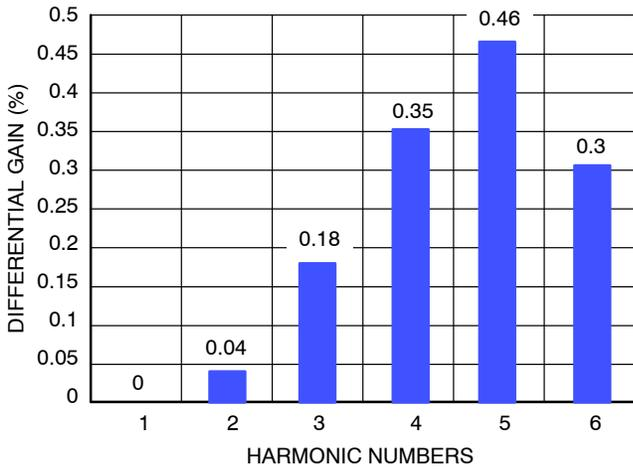
Figure 10. Differential Gain (NTSC 5 Steps Input Signal)
