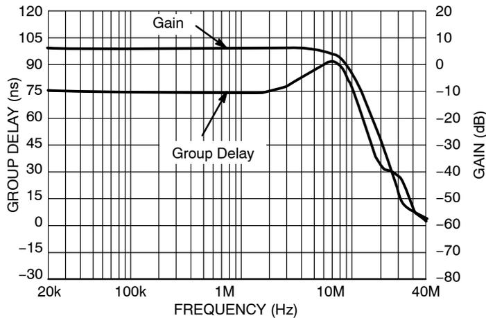
Figure 12. Normalized Frequency Response and Group Delay vs. Frequency
