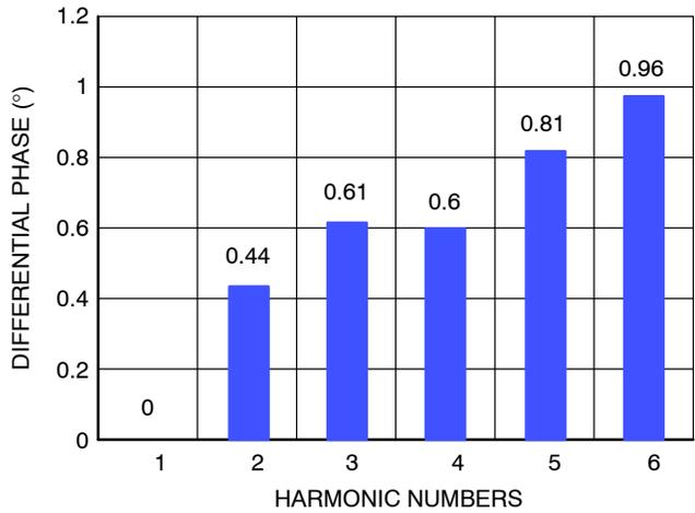
Figure 11. Differential Phase (NTSC 5 Steps Input Signal)
