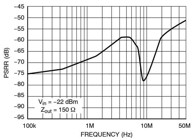
Figure 8. PSRR vs. Frequency (Bypass Capacitor)
