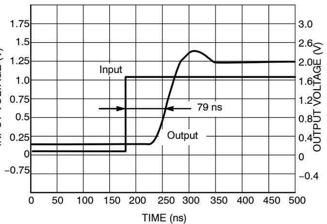
Figure 6. Propagation Delay
