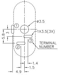
Recommended PCB Layout Top View
