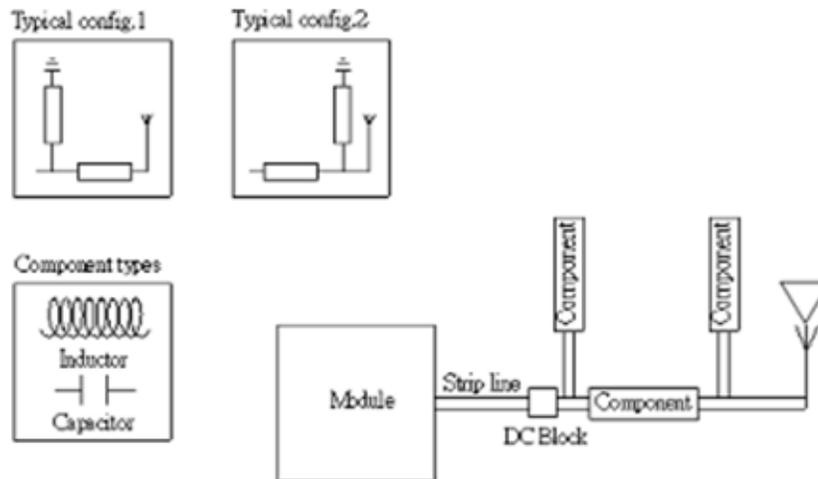
Matching should be considered using a Pi network where 1, 2 or 3 components could be used. This shall be matched to the transmission line and the ground plane in the design.
