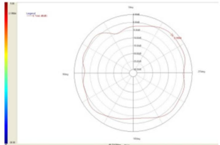
2D Radiation Pattern X-Y Plane 5550MHz
