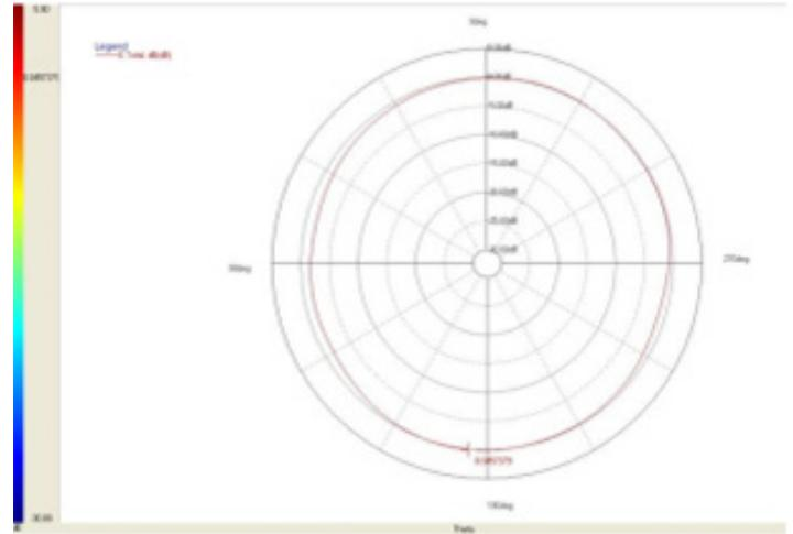
2D Radiation Pattern X-Y Plane 2450MHz
