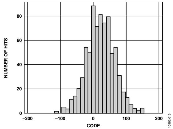
Figure 13. Channel Offset Distribution (Gain = 35 dB)
