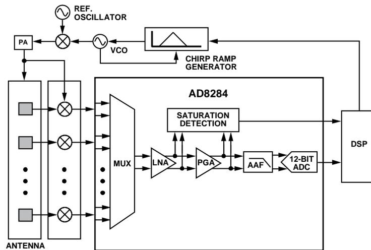
Figure 14. Simplified Block Diagram, HSR-FMCW Radar System
