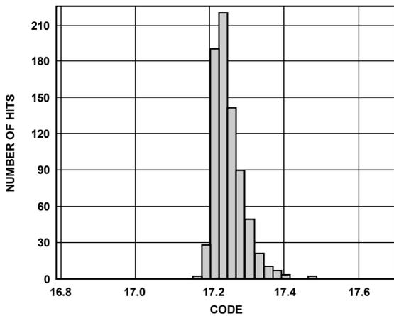
Figure 5. Gain Histogram (Gain = 17 dB)
