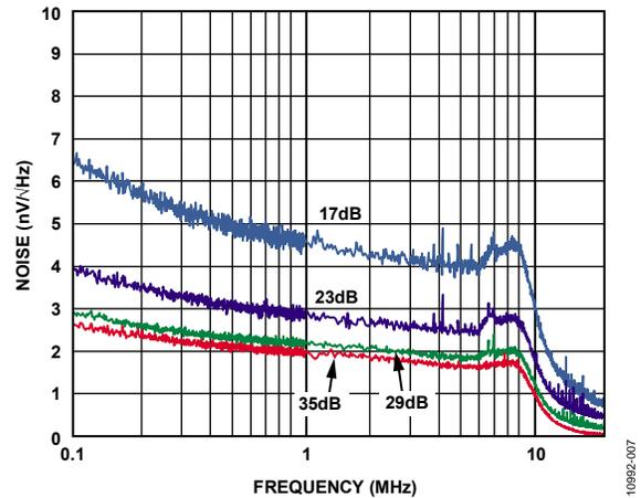
Figure 7. Short-Circuit Input Referred Noise vs. Frequency
