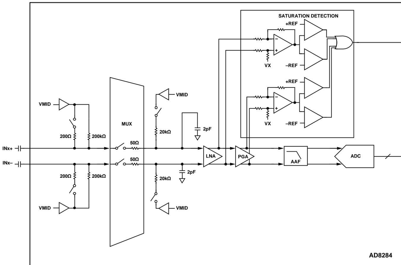
Figure 16. Simplified Block Diagram of the Analog Channel
