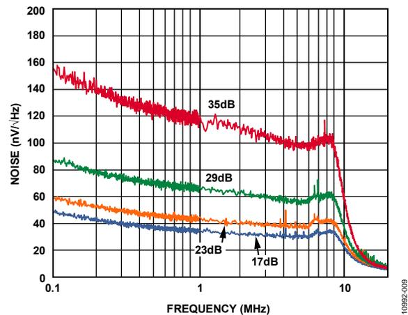
Figure 9. Short-Circuit Output Referred Noise vs. Frequency
