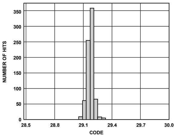
Figure 6. Gain Histogram (Gain = 29 dB)
