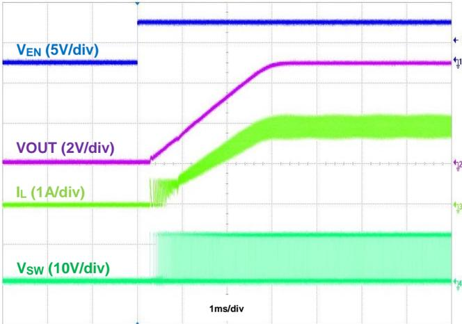
Figure 21. Startup Using EN, IOUT = 2A
