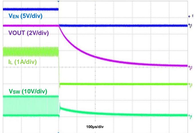
Figure 22. Shutdown Using EN, IOUT = 2A
