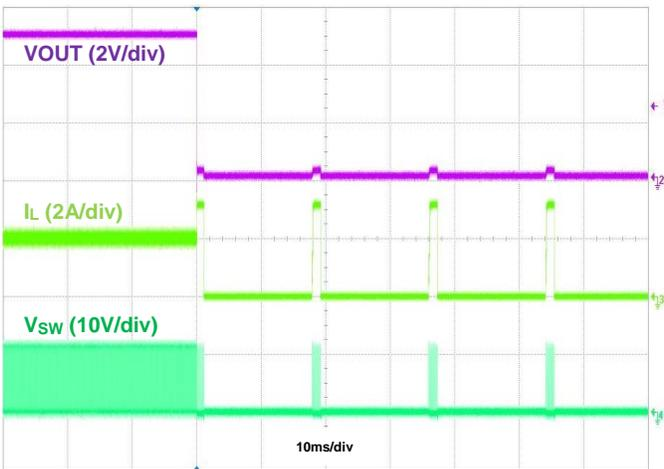
Figure 23. Output Short Protection, IOUT = 2A
