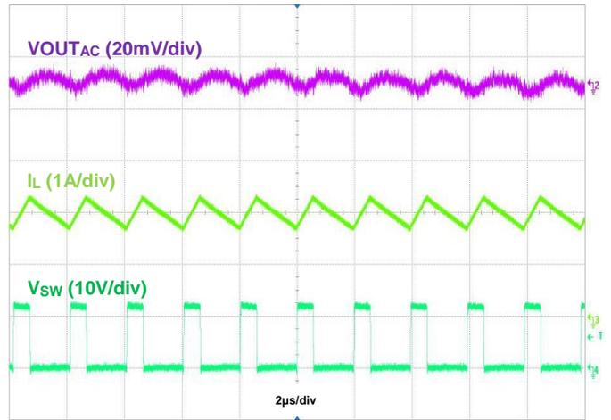
Figure 17. Output Voltage Ripple,  $V_{OUT} = 3.3\text{V}$ ,  $I_{OUT} = 2\text{A}$
