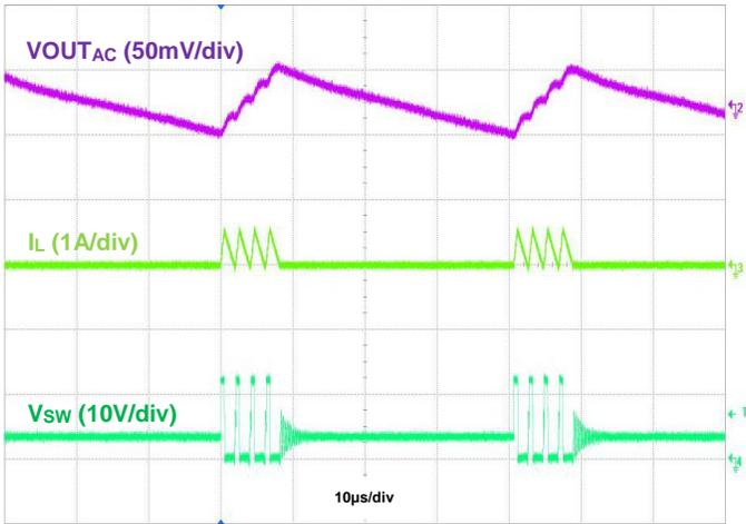
Figure 16. Output Voltage Ripple,  $V_{OUT} = 3.3\text{V}$ ,  $I_{OUT} = 50\text{mA}$
