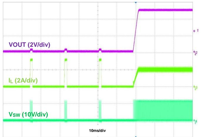
Figure 24. Output Short Recovery, IOUT = 2A
