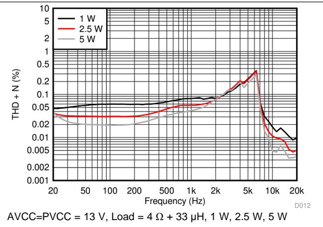
Figure 12. Total Harmonic Distortion + Noise vs Frequency (PBTL)
