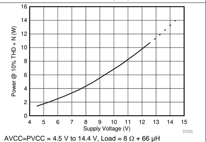
Figure 6. Output Power vs Supply Voltage (BTL)
