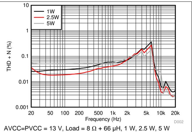
Figure 2. Total Harmonic Distortion vs Frequency (BTL)
