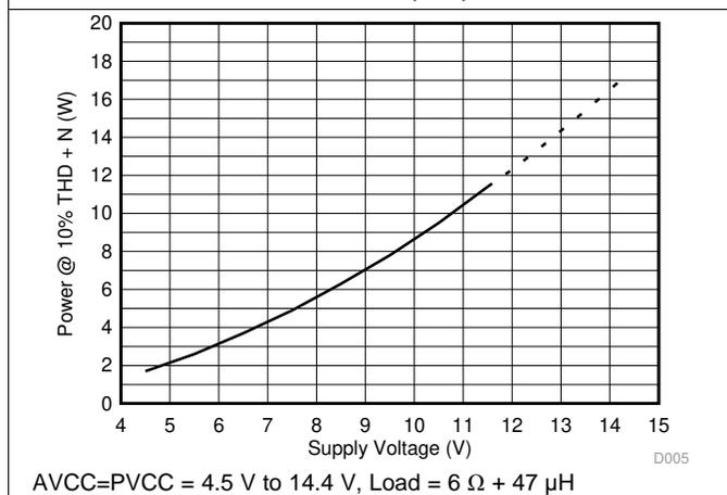
Figure 5. Output Power vs Supply Voltage (BTL)
