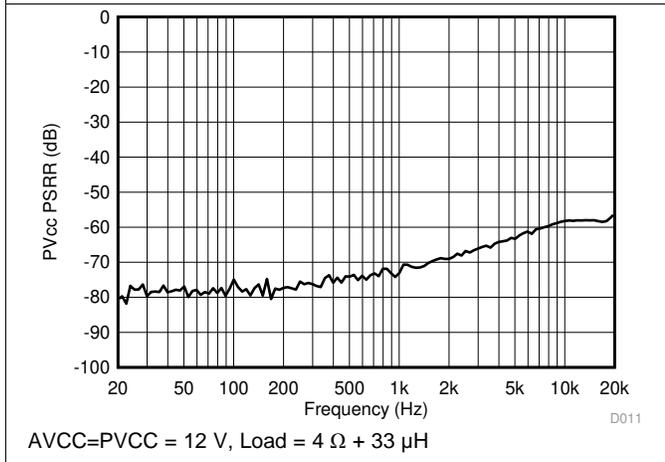
Figure 11. Supply Ripple Rejection Ratio vs Frequency (BTL)
