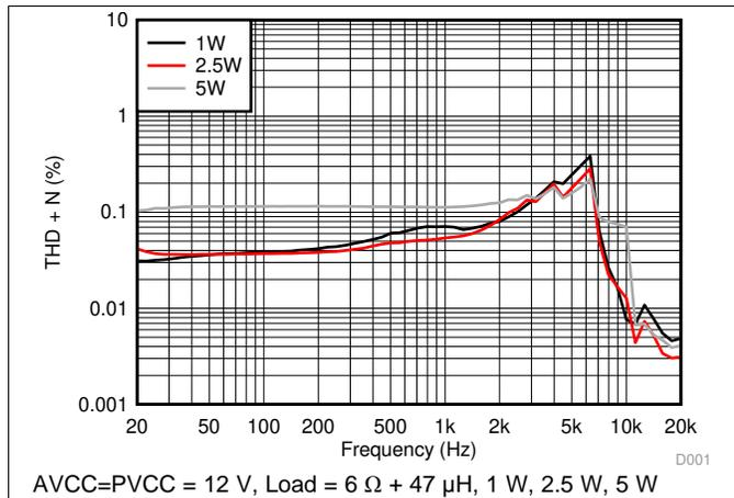
Figure 1. Total Harmonic Distortion vs Frequency (BTL)
