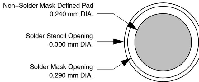
Figure 10. Recommended Non-Solder Mask Defined Pad Illustration
