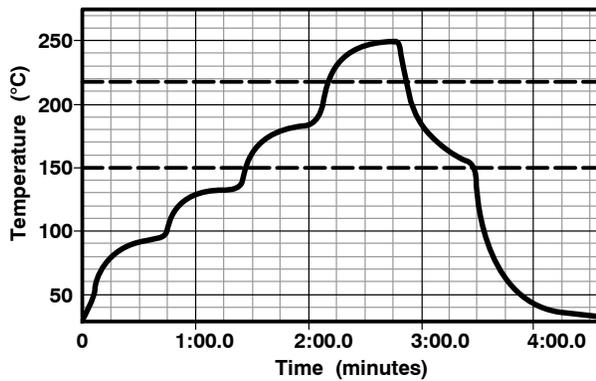
Figure 11. Lead-free (SnAgCu) Solder Ball Reflow Profile
