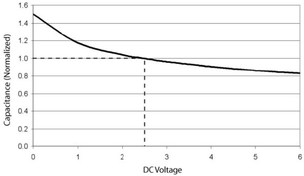
Figure 9. Filter Capacitance vs. Input Voltage
