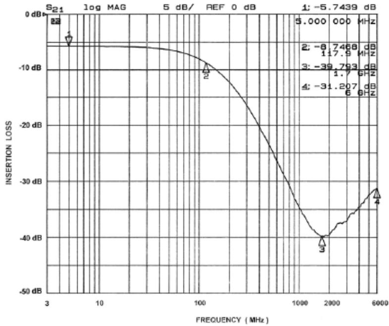
Figure 1. Insertion Loss vs. Frequency (A1-C1 to GND B1)
