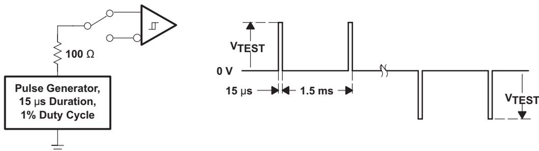
Figure 10. Test Circuit and Waveform, Transient Over-Voltage Test
