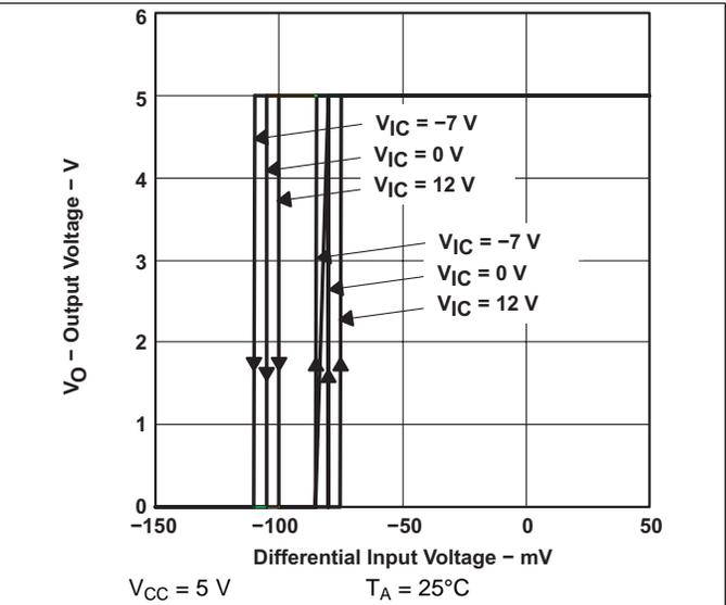
Figure 3. Output Voltage vs Differential Input Voltage
