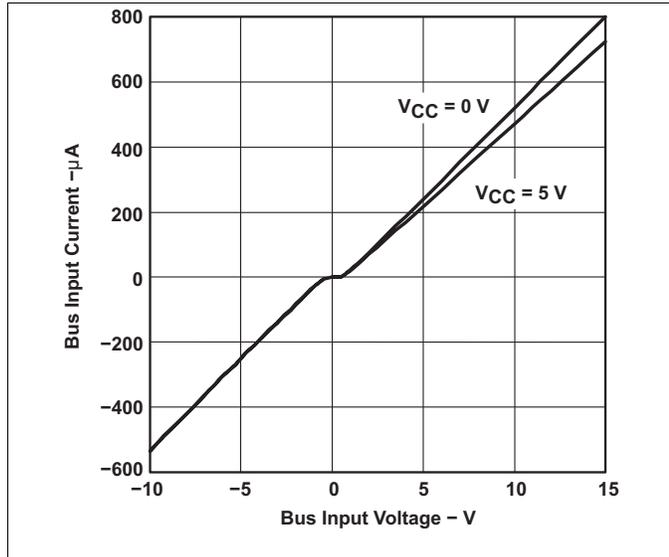
Figure 2. Bus Input Current vs Bus Input Voltage
