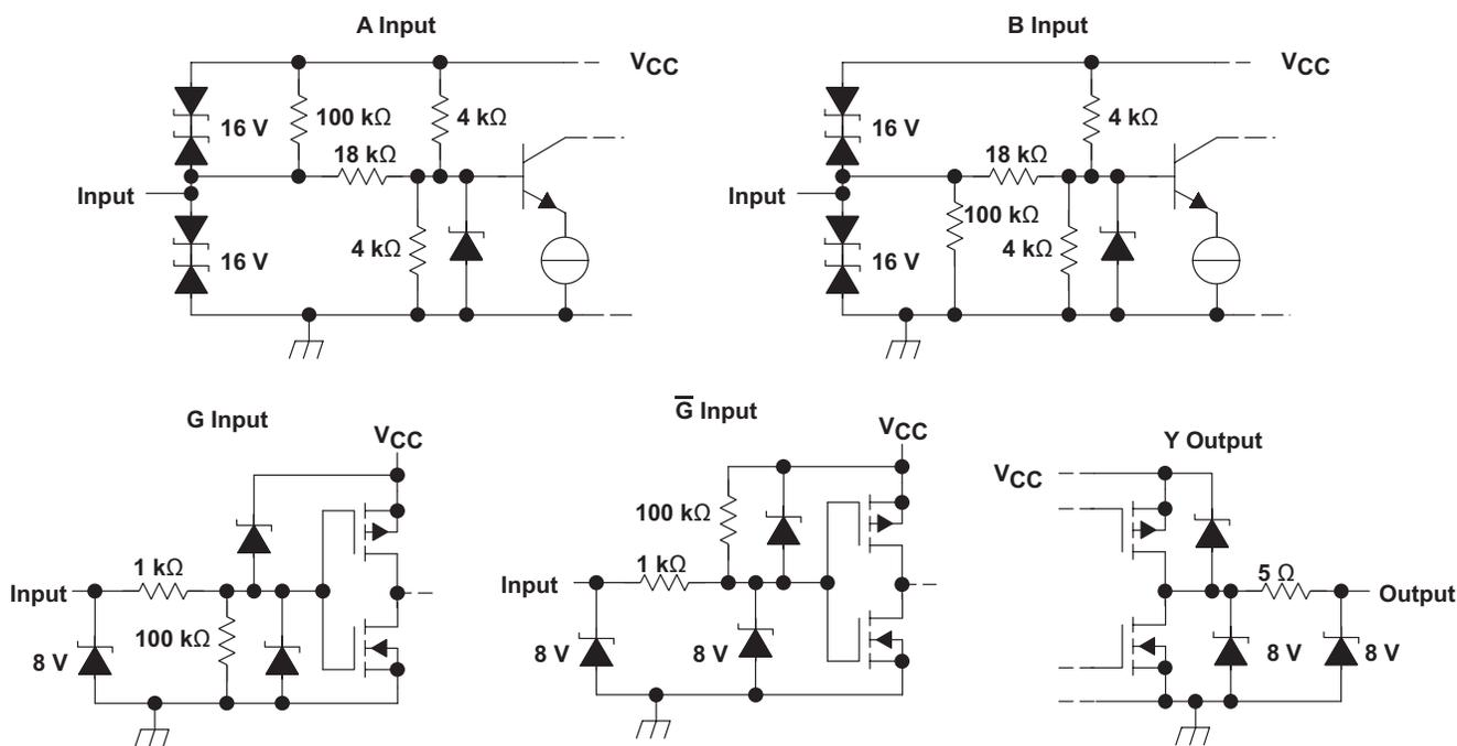
Figure 11. Equivalent Input and Output Schematic Diagrams
