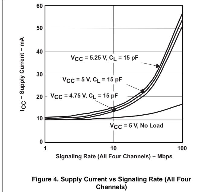
Figure 4. Supply Current vs Signaling Rate (All Four Channels)
