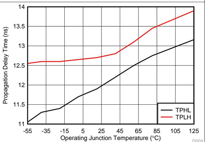
Figure 5. Propagation Delay Time vs Free-Air Temperature
