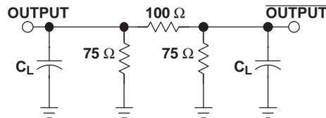
Figure 4. Driver Test Circuits, 3.3-V Nominal Supplies
