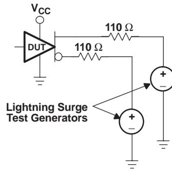
Note: Surges may be applied simultaneously, but never in opposite polarities. Surge test pulses have  $t_r = t_f = 2 \mu s$ , pulse width =  $7 \mu s$  (50% points), and period = 250 ms.
