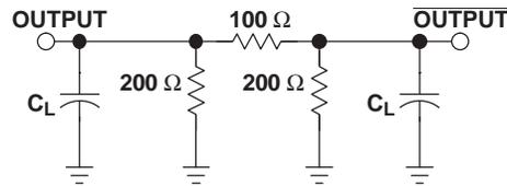
Figure 3. Driver Test Circuits, 5-V Nominal Supplies
