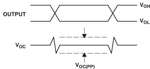
Note: All input pulses are supplied by a generator having the following characteristics:  $t_r$  or  $t_f = 1$  ns, pulse repetition rate (PRR) = 0.25 Mbps, pulse width =  $500 \pm 10$  ns.  $C_p$  includes the instrumentation and fixture capacitance within 0,06 m of the D.U.T. The measurement of  $V_{OC(PP)}$  is made on test equipment with a  $-3$  dB bandwidth of at least 1 GHz.
