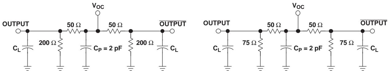
Note:  $V_{OC(PP)}$  load circuit for 5-V nominal supplies.
