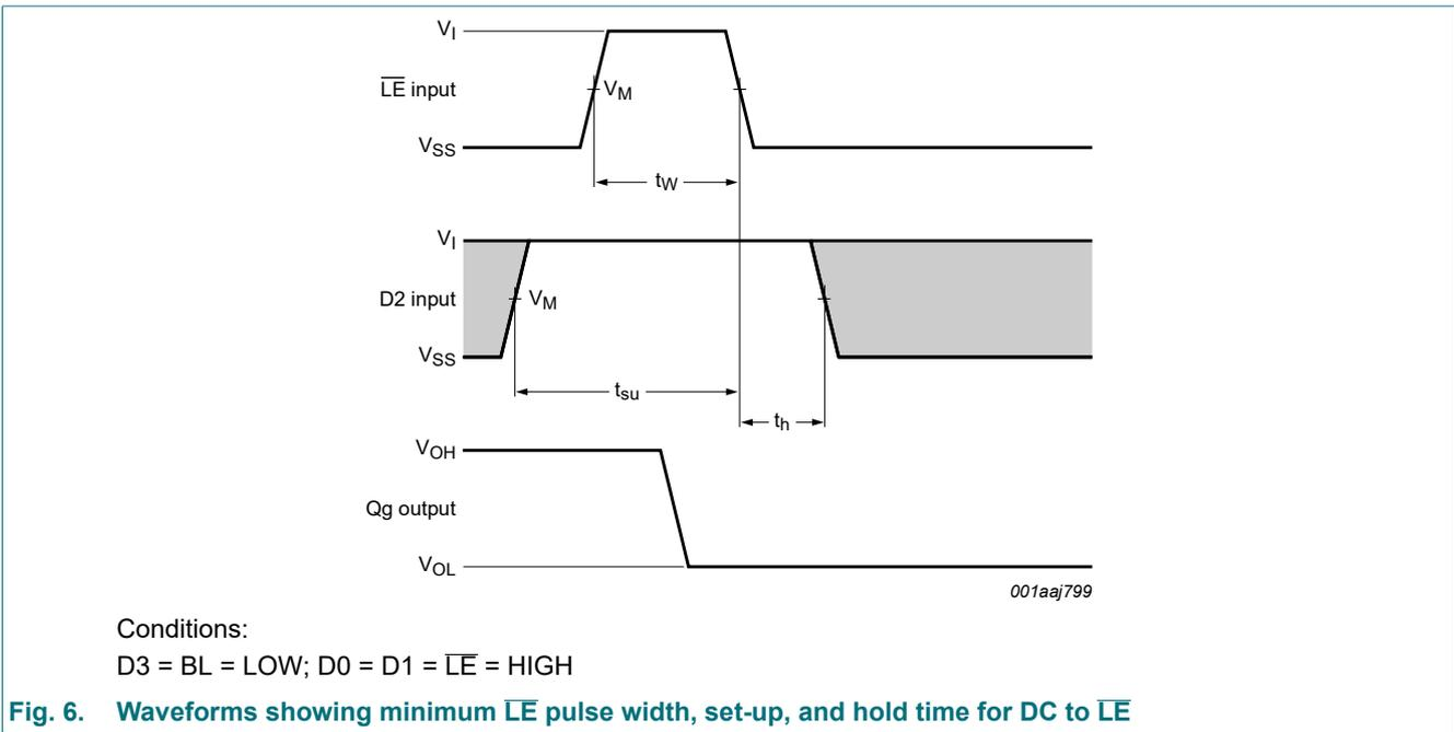
Fig. 6. Waveforms showing minimum LE pulse width, set-up, and hold time for DC to LE
