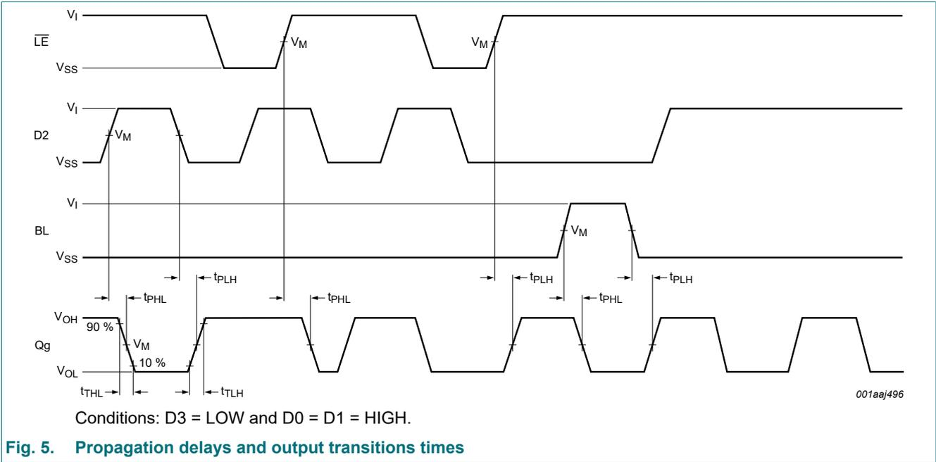
Fig. 5. Propagation delays and output transitions times
