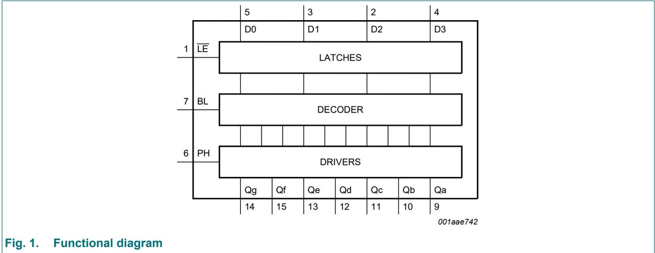
Fig. 1. Functional diagram
