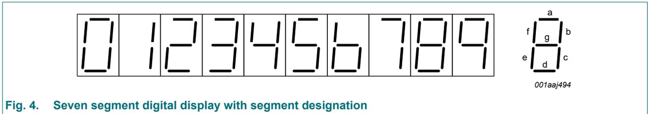
**Fig. 4. Seven segment digital display with segment designation**
